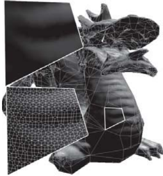
Fig. 3. Close-up view of one normal map of the dragon, shown at a coarse level (16K) and the finest level (225K). The finest level view shows the wireframe projected onto the normal map extracted for the coarse mesh. The normal map shown is approximately 30 by 30 texels, closely matching the resolution of the finest level mesh.
