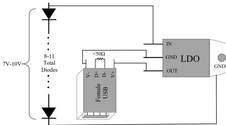
Figure 3: A circuit diagram of the ISEC phone charging circuit connected to the ISEC's diode chain.
