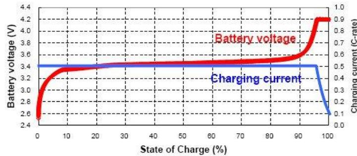
Figure 4: Charging Diagram of a single cell LiFe battery
