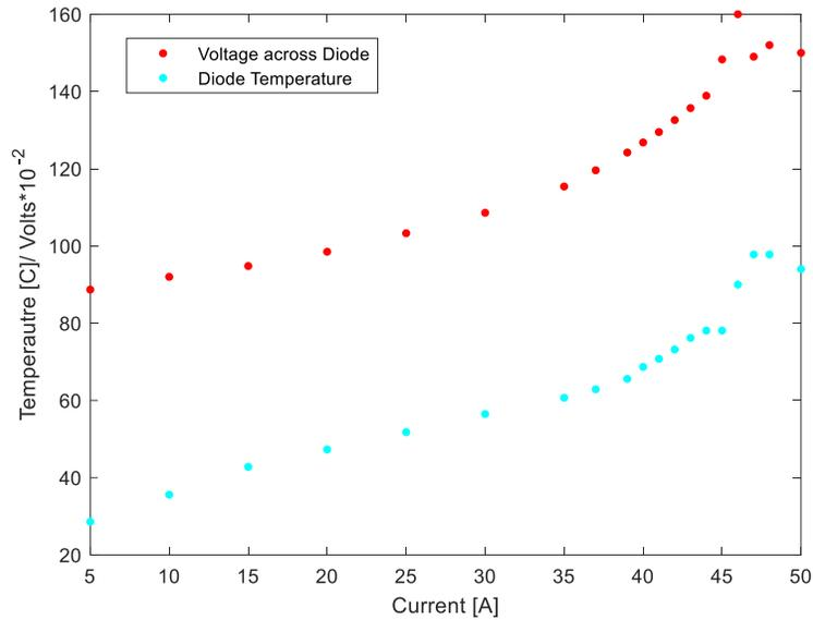
Figure 7: A graph of diode temperature and voltage drop vs current from a water-diode test. Data collection ended with diode failure. Note the changing rates in the increasing voltage drop across the diodes.
