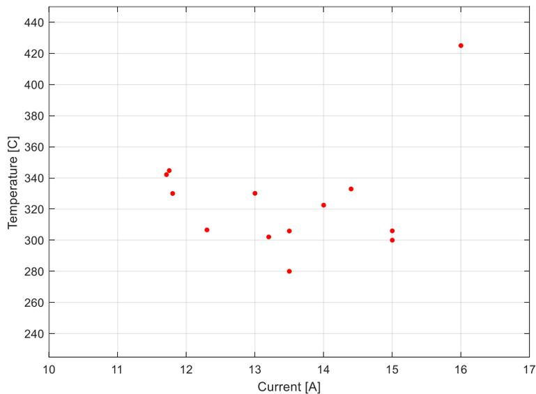
Figure 8: Failure point from multiple diode failure tests. Each point represents the failure of a diode at a given current and corresponding temperature. This data was taken in collaboration with Andre Li.
