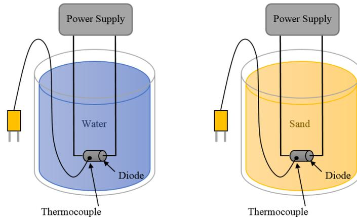
*Figure 1 (left) and Figure 2 (right):* The testing setup used in the previously described experiments. Both setups had a diode directly connected to a high current power supply and a thermocouple directly attached to diode body to record temperature. Figure 1 shows a diode submerged in distilled water while Figure 2 shows a diode buried in sand.
