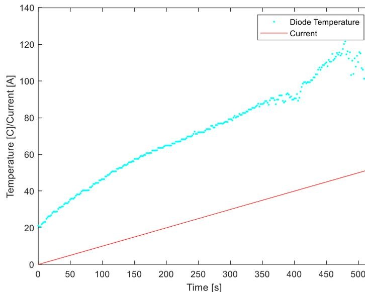
Figure 6: A graph of diode temperature and current vs time from a water-diode test. Data collection ended with diode failure.
