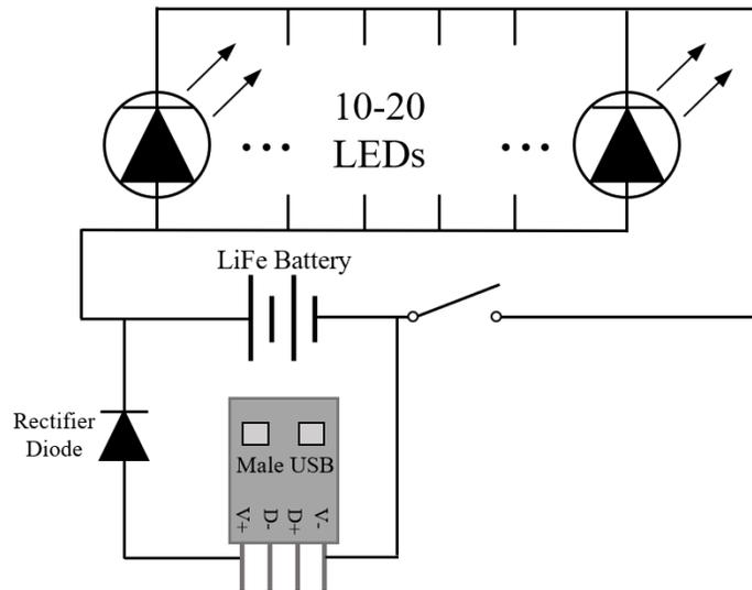
Figure 5: Circuit diagram of LED lighting system, including the LiFe battery and recharging system.
