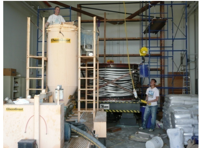
Figure 3. Testing platform showing the shake table with the flexible wall barrel. The flexible wall barrel is composed of the four corner posts with universal joints at the top and bottom, the top and bottom rings, and the barrel wall. The wall is composed of a 6.4 mm thick rubber membrane which is confined by 45 mm wide Kevlar straps spaced on center every 60 mm. The (yellow) mixer on the left is used to mix the large volumes of model soil (composed of kaolinite, bentonite, fly ash, and water).
