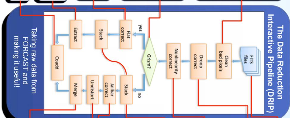
Flexible Image Transport System (FITS) files are what FORCAST outputs as raw data and is the format of choice for astronomers.
