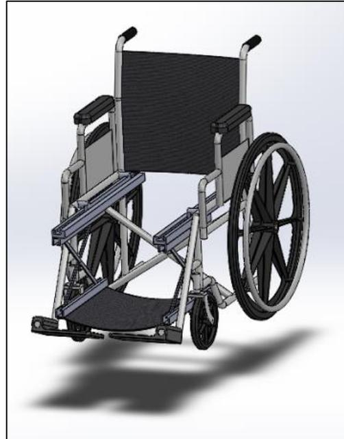
Figure 6: Prototype when seat is down and forward
