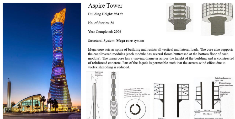
Figure 2 – Aspire Tower Case Study
