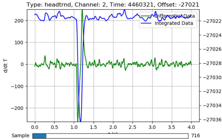
Figure 5: Sample of a noise pulse with an anomaly. Although there appears to be some sort of pulse at 1 second which would constitute a signal capture, the pulse is inverted and slightly after 1 second which clarifies that this is in fact a noise capture.
