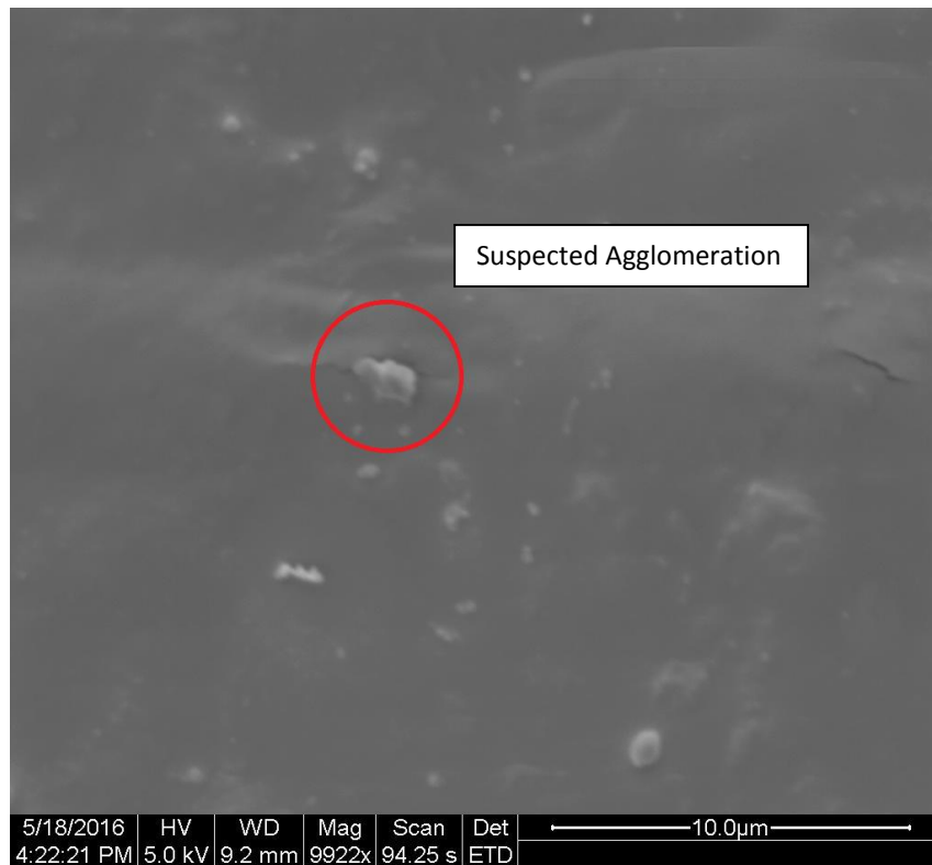
Figure 9 – A suspected agglomeration of NCC particles in the 3 wt. % NCC sample. These agglomerations prevent the composite from having maximum mechanical strength and stiffness. Similar particles were found in the 5 wt. % samples.
