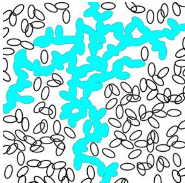
Figure 6 – A diagram depicting a quasi-continuous fiber made from particles shown in blue. These networks help support a load. White particles are not interconnected and thus do not form networks.
