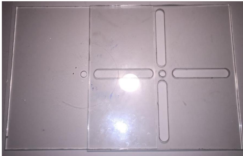
Figure 7: Acrylic 12"x12"x0.220". The right piece is to act as a top and is slotted for accessibility to the wire to put on epoxy or fix layout of wire. The left piece is to act as a bottom that fits the copper wire.
