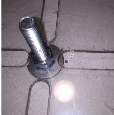
Figure 8: Acrylic assembled with \frac{1}{2} "-13 threaded bolt, \frac{1}{2} "-13 nut, and washer as a spacer. (A) and (B) from Figure 1 are used as a top and bottom piece respectively.
