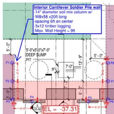
Figure 5: Drawings detailing shoring plan including layout of soldier piles and lagging
