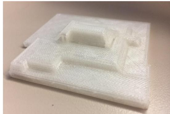
*Figures 3 and 4: 3D printed model of the base of slab excavation used on the project*
