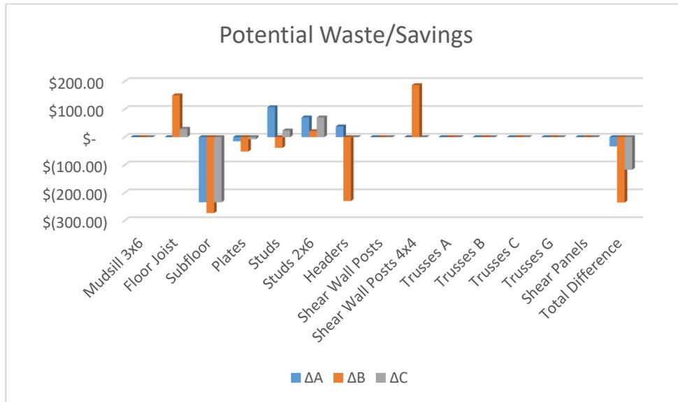
Figure 5: Potential Waste/Savings with ArchiCAD as a Constant
