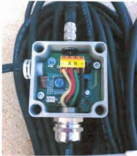
Figure 24: Breather Box Configuration for water level sensor (Kloepper, 2014)
