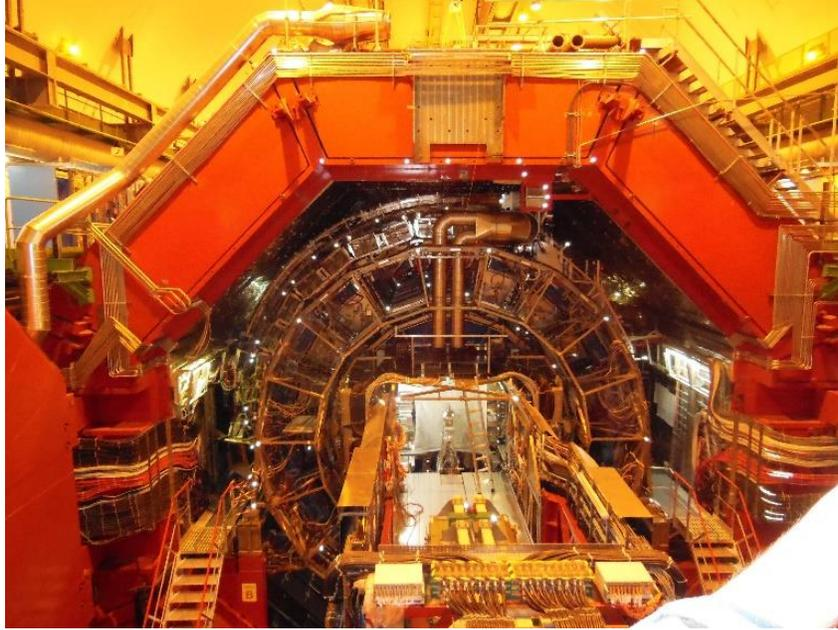
Figure 4: (Top) Picture of ALICE Detector with camera flash on to illustrate where each particle detector is located and to check their respective alignment. Source: <http://aliceinfo.cern.ch/Public/en/Chapter2/Chap2InsideAlice-en.html>
