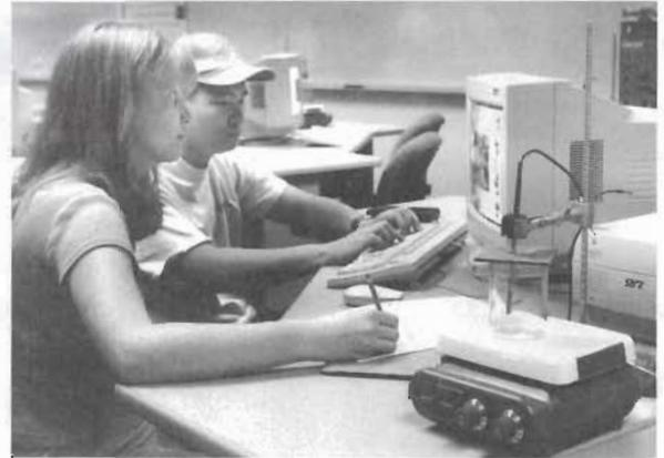
Mathematics, where lectures and labs are integrated and pairs of computers are hard-wired to lab equipment. Shown here (right foreground) is a computer-interfaced temperature probe for monitoring acidity, pressure, and electrical changes during chemical processes; a hot plate/stirrer is used for mixing samples. **CP** (Photo by Doug Allen)
