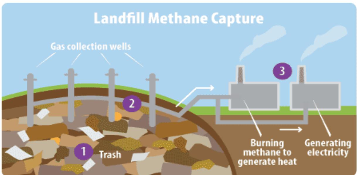
Fig 8 Capturing methane to convert into energy. "Landfill Methane Capture". Illustration. 21 June 2013. Methane Capture and Use. EPA. Web. 07 Sept. 2013.
