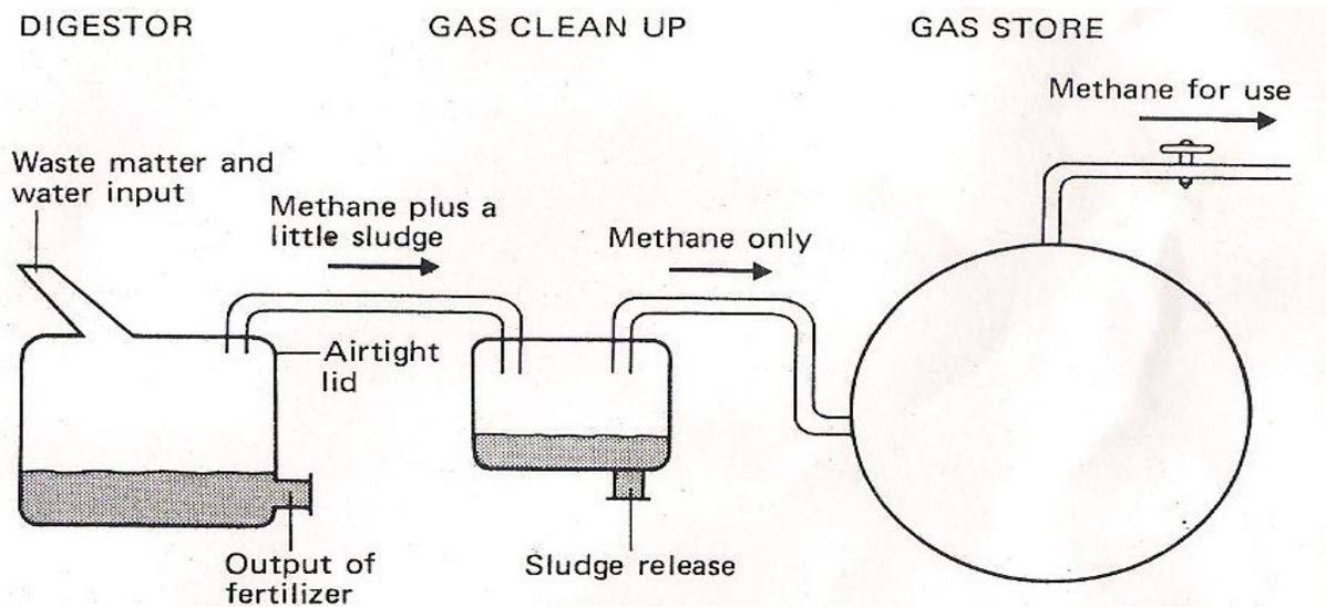
Fig. 7 Methane digester. "Basic Methane Production and Storage". Graph. 1979. *Your Solar Energy Home : Including Wind and Methane Applications*. Pergamon Press. Print. Methane gasses are already being successfully produced as useable commercial energy
