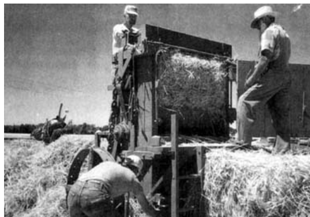
Figure 2. The Petaluma Hay Press. Shown packaging alfalfa into bales. Picture courtesy of Farm Collector.
