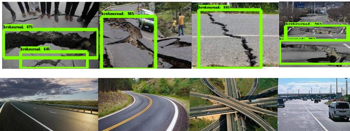
Figure 7. Output images from deep learning classifier for the set of images from Figure 6. *Note: If the algorithm does not detect damage, the original image will remain unchanged as seen with images of no cracking.*
