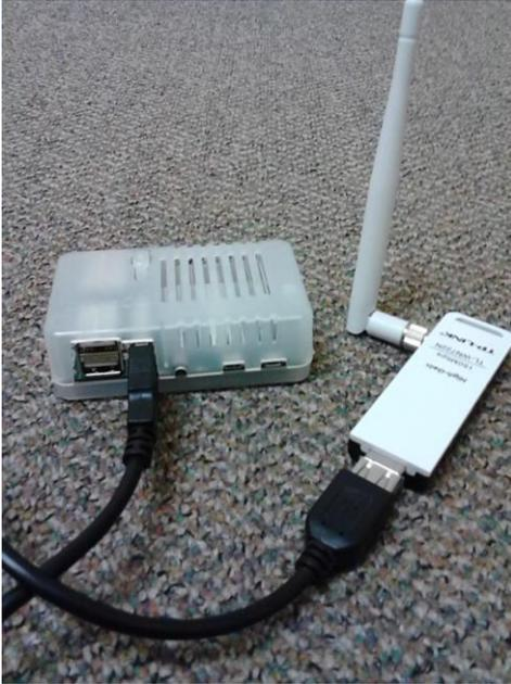
2. Connect the device to your **Home Router** through an Ethernet Cable.
