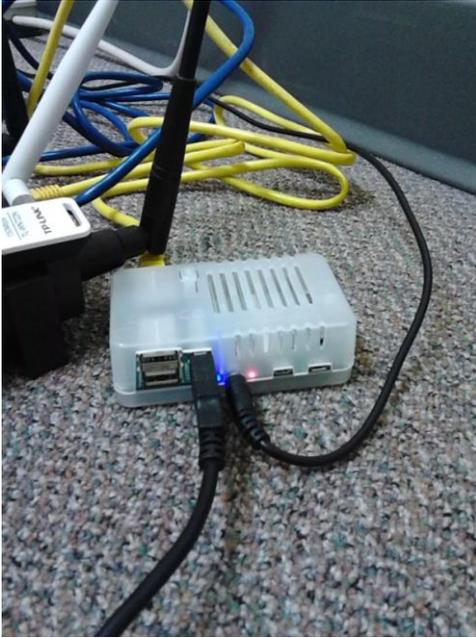
4. A **blinking blue light** indicates that the device is running. Wait for about **two minutes** to let the system boot up. Then, go to **System Setup** for configuring the system.
