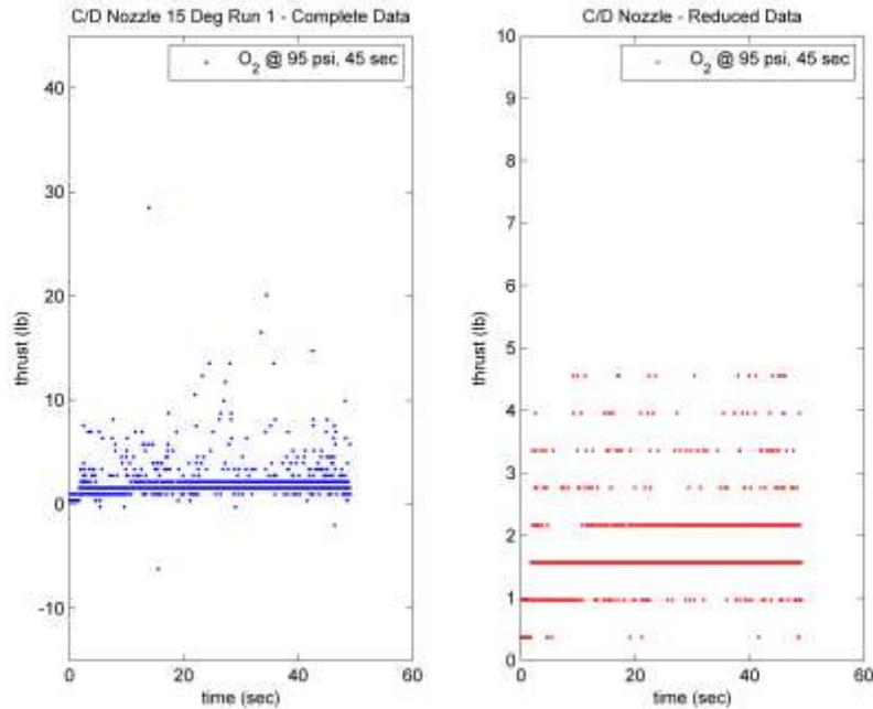
Figure 4. Thrust of 15 Degree Nozzle for the First Day. Right Plot Shows Reduced Data
