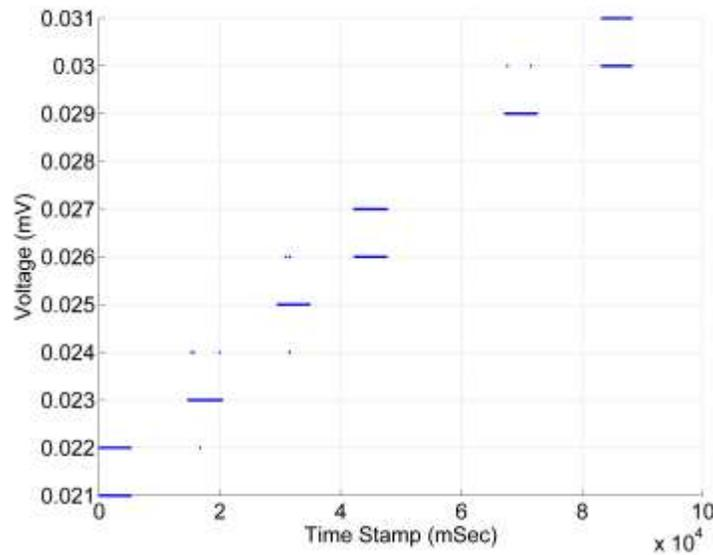
Figure 3. Calibration data used to create a linear regression line that gave the corresponding force for a given voltage.
