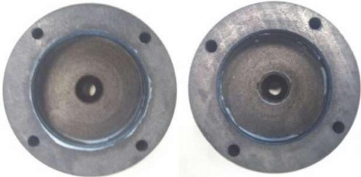
**Figure 7. 15-Degree Nozzle (left) and 30-Degree Nozzle (right).**
