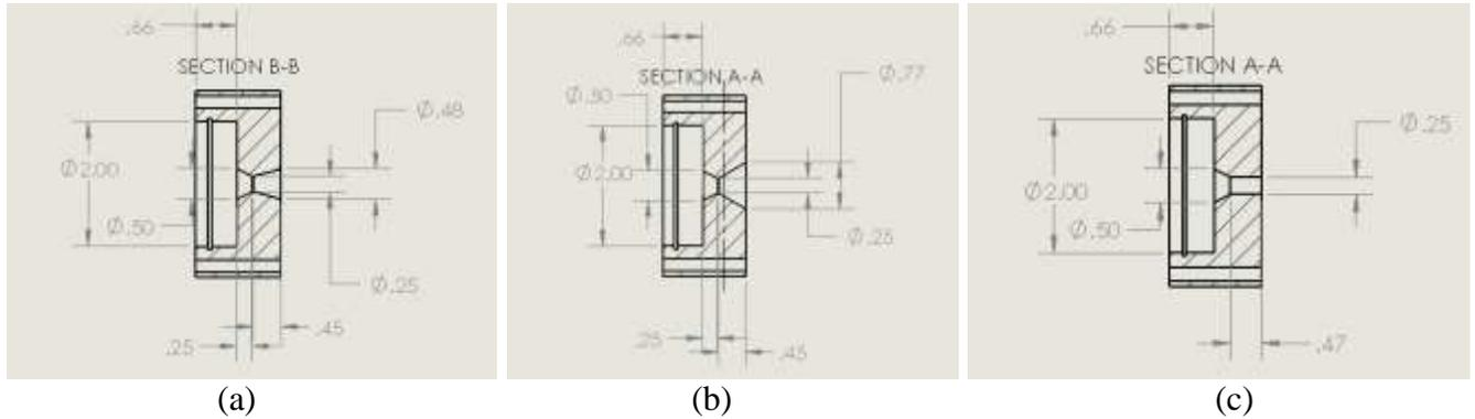
Figure 2. (a) 15 Degree Nozzle (b) 30 Degree Nozzle (c) Hole nozzle
