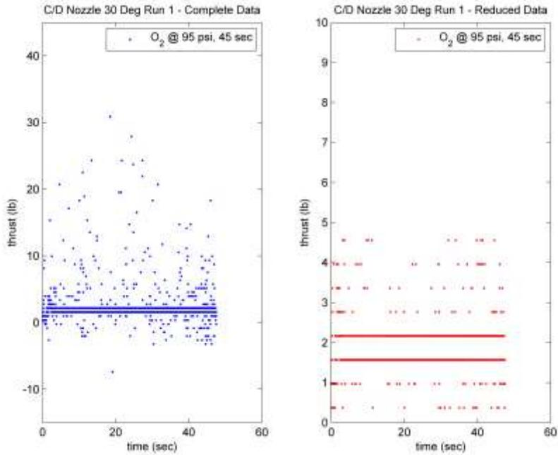
Figure 6. Thrust of 30 Degree Nozzle for the First Day. Right Plot Shows Reduced Data
