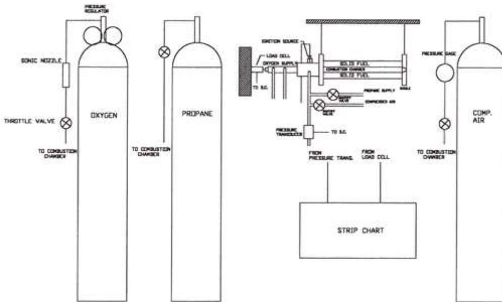
Figure 1 Hybrid Rocket Setup<sup>1</sup>
