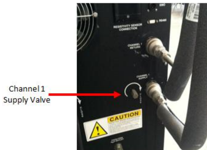
Figure 22. Channel 1 Supply and Return
