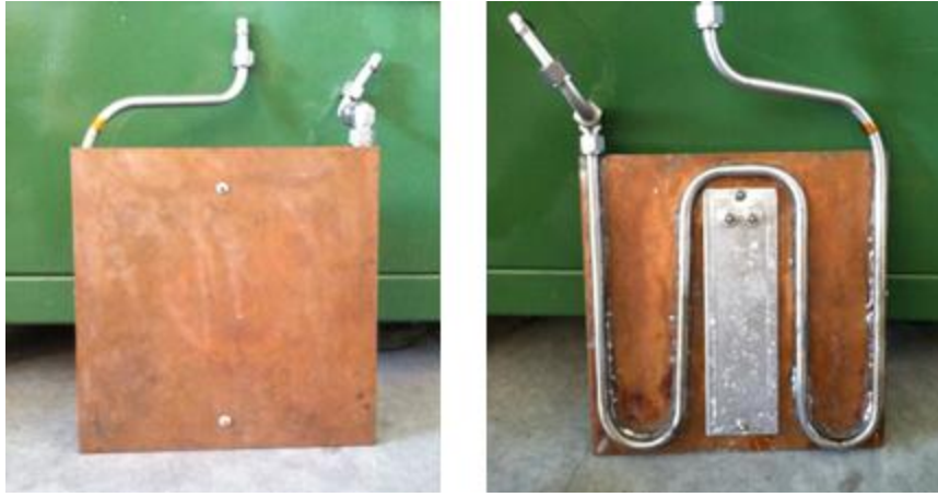
Figure 2. Copper Plate. Left image is the top of the plate and faces the ceiling when in use. Right image is the underside of the plate. The gray pipe runs fluid under the plate.
