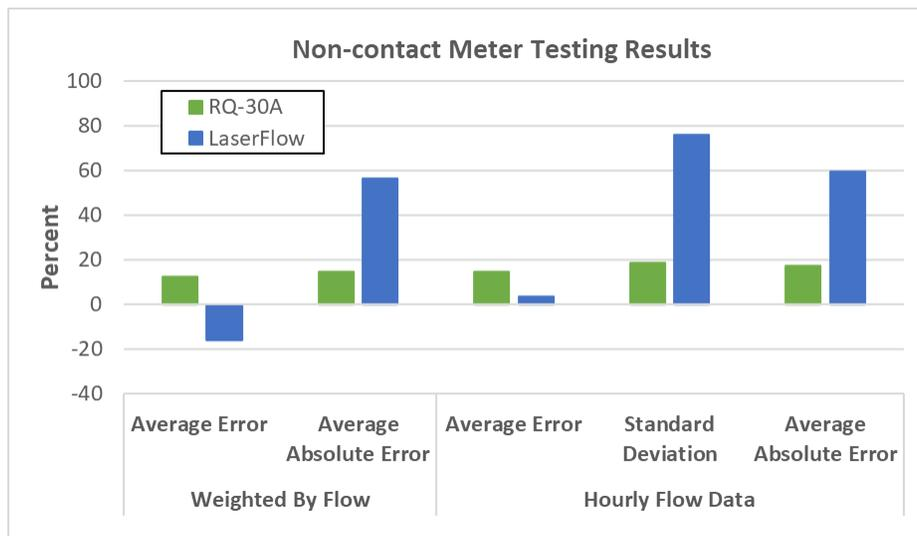
Figure 4. Results of non-contact meter testing at PID
