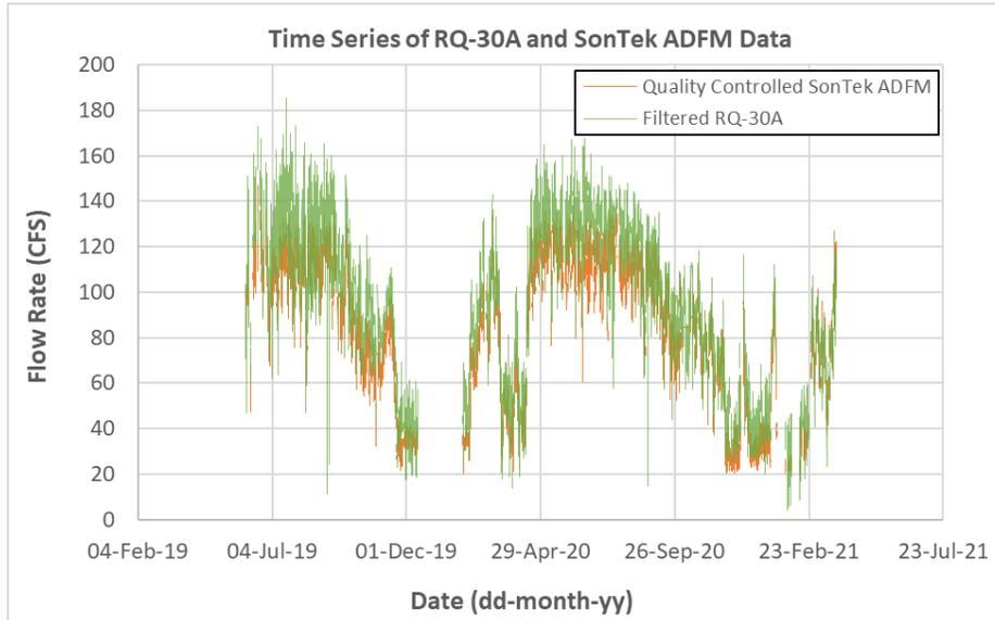
Figure 7. Hourly RQ-30A and SonTek ADFM flow rate data
