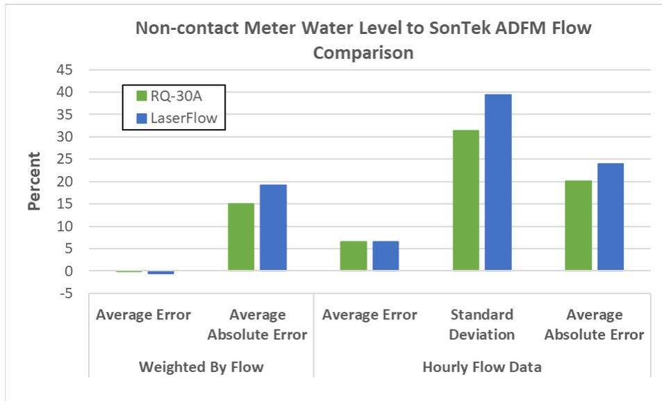
Figure 11. Results of using the non-contact meter water level measurement to predict the flow
