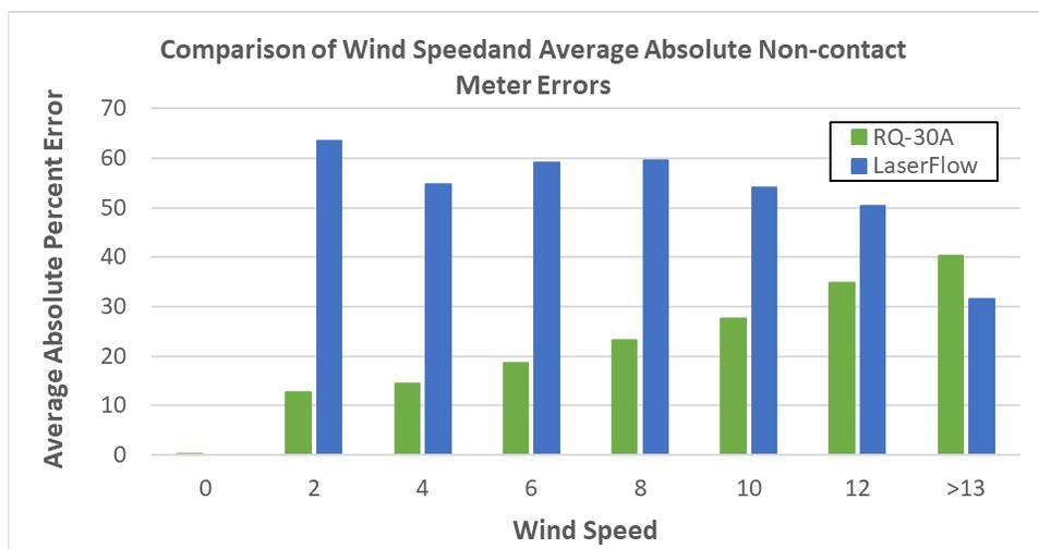
Figure 10. Non-contact meter average absolute percent errors for each wind speed
