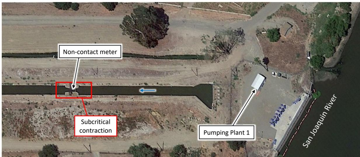
**Figure 2. Aerial map view of PID Main Canal and non-contact meter installation**
