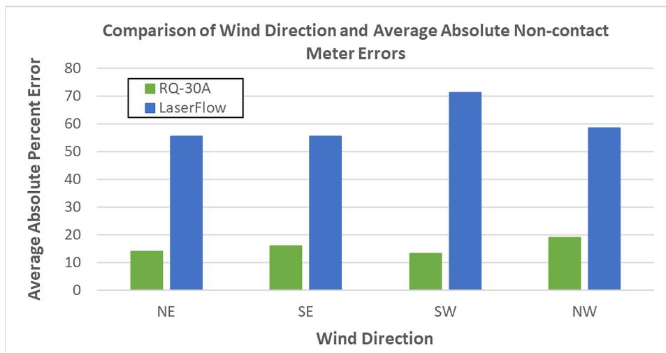
Figure 9. Non-contact meter average absolute percent errors for each wind direction
