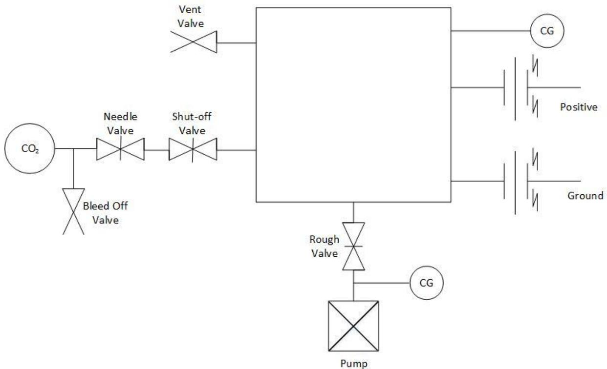
**Figure 2. Cal Poly Student Chamber I vacuum schematic.** *CG stands for convectron gauge.*
