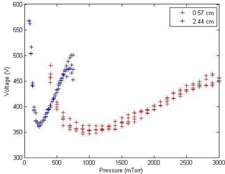
Figure 3. Voltage versus pressure in air. Unaltered measurements.
