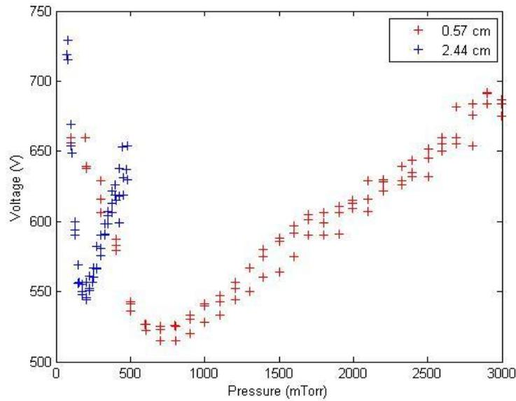
**Figure 5. Voltage versus pressure in CO<sub>2</sub>. Unaltered measurements.**
