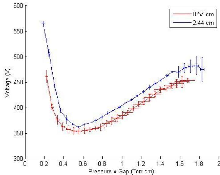
**Figure 4. Paschen Curves in air.** *The averaged data with error.*
