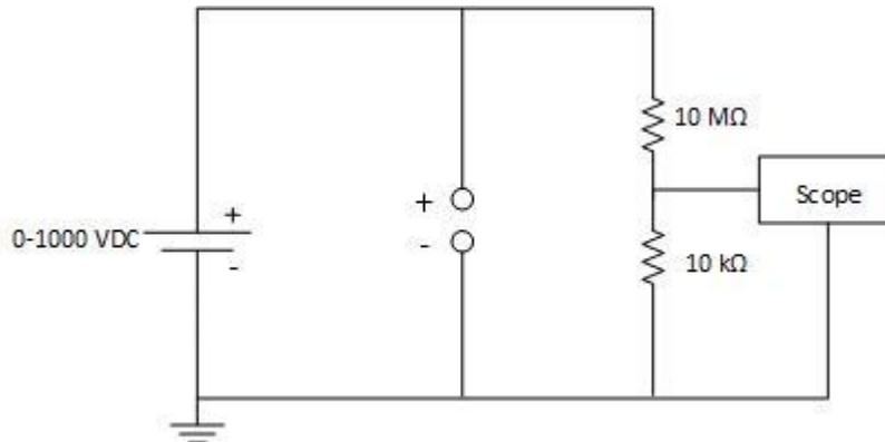
Figure 1. The Cal Poly Paschen Breakdown Apparatus electrical schematic.
