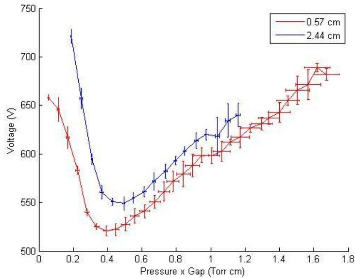
**Figure 6. Paschen Curves in CO<sub>2</sub>. Note the difference in the minimum breakdown potentials between the two gap distances.**
