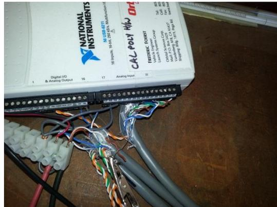
**Figure 9. DAQ Wiring.** *The wiring from the shielded cable to the DAQ.*
