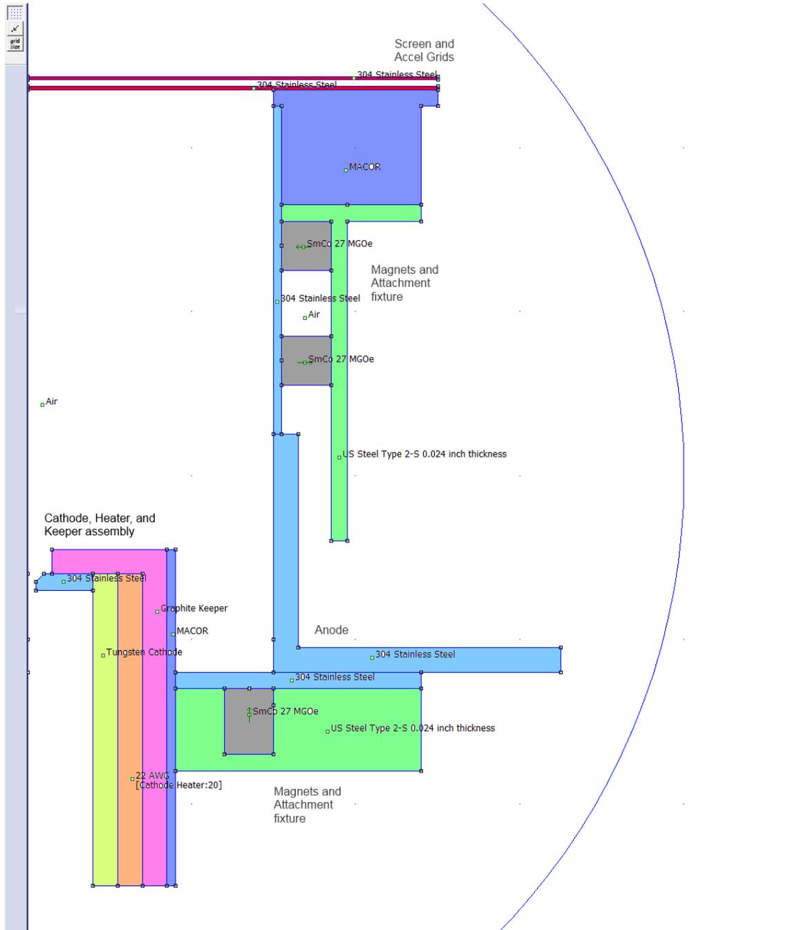
**Figure 4: FEMM model of the thruster structure colored and annotated. Also shown are the placement and orientation of the permanent magnets.**
