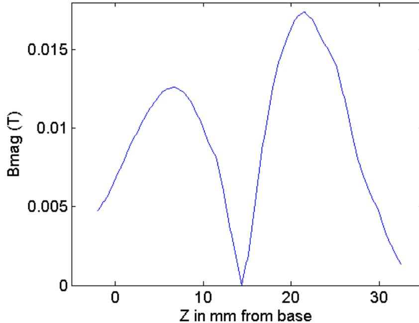
**Figure 9: Magnetic field strength in Tesla along the centerline of the discharge chamber**
