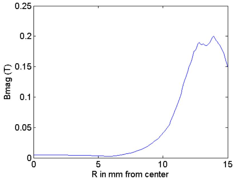
**Figure 8: Magnetic field strength in Tesla along the bottom edge of the discharge chamber, along the anode base and intersecting the cathode assembly**
