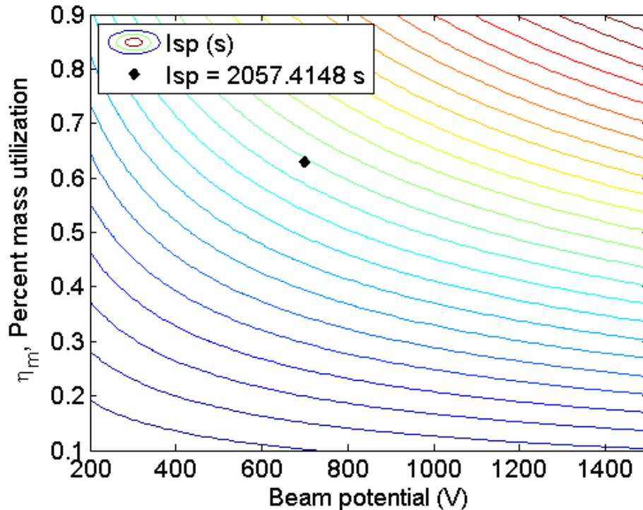
**Figure 12: Theoretical  $I_{sp}$  as a function of beam potential and percent mass utilization**
