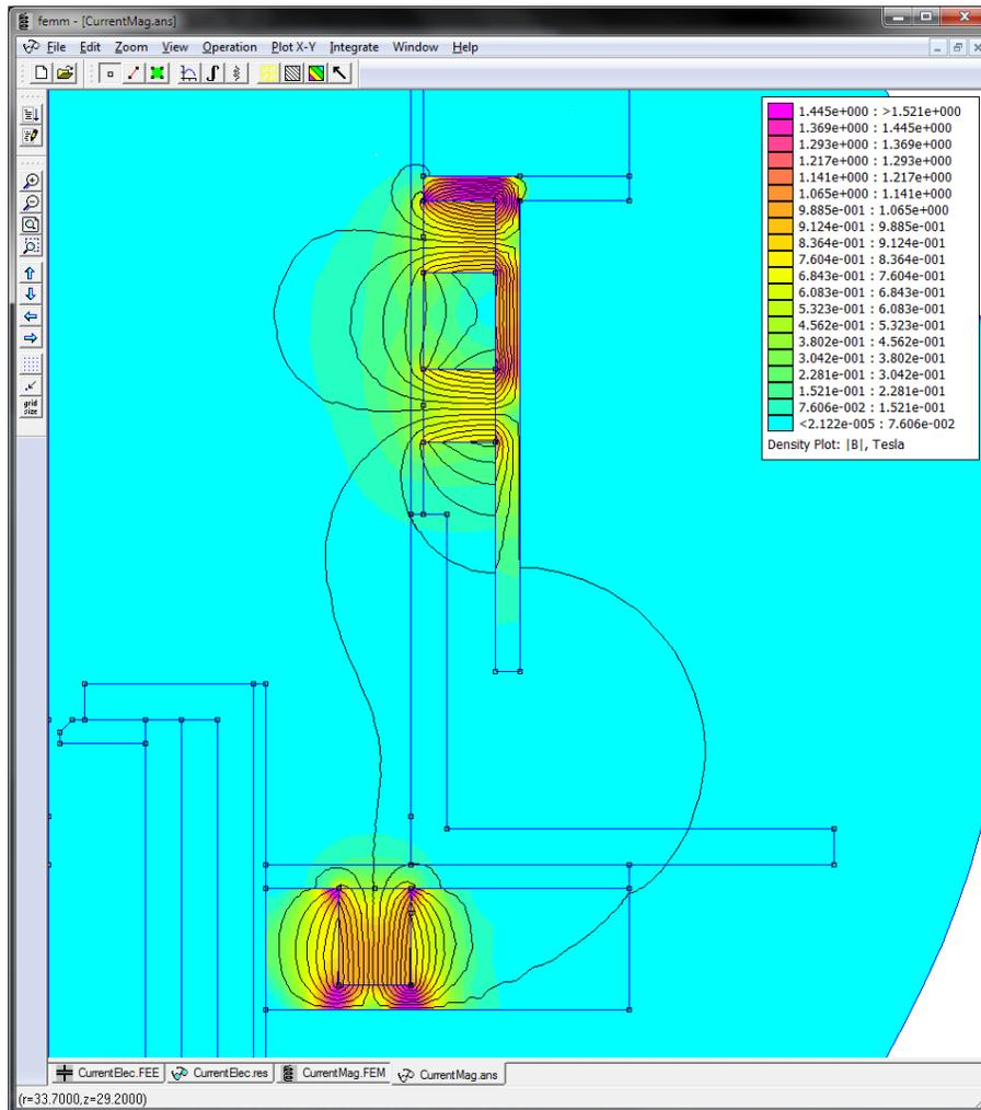
**Figure 5: Using the FEMM solver to display the magnetic field within the entire thruster.**
