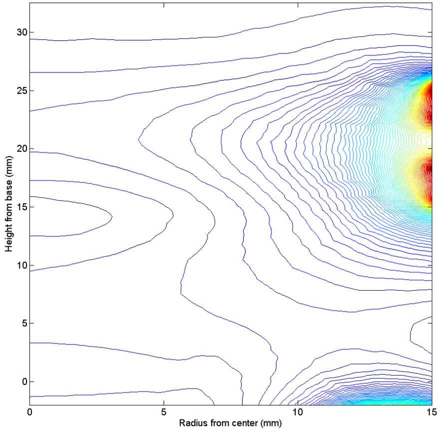
**Figure 6: The magnetic strength within the discharge chamber from all magnetic sources.**
