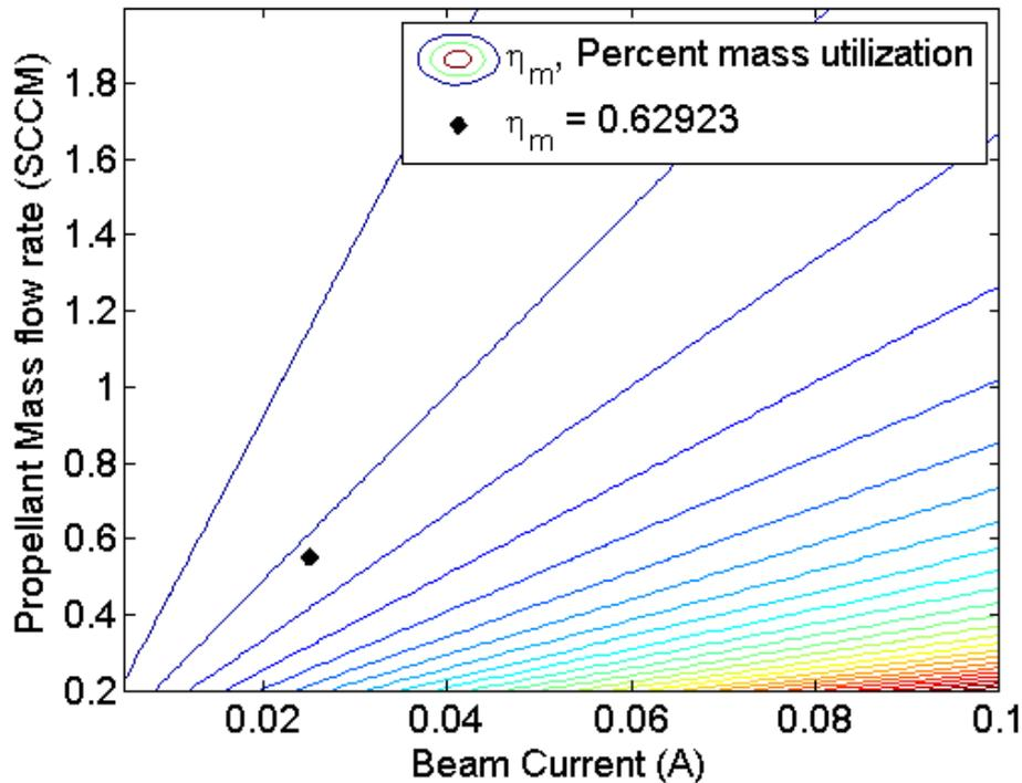
**Figure 11: Percent mass utilization as a function of beam current and propellant mass flow rate**
