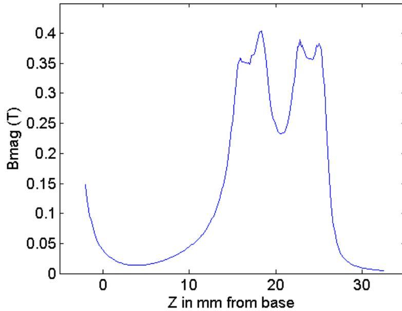
**Figure 7: Magnetic field strength in Tesla along the right edge of the discharge chamber, the anode wall**
