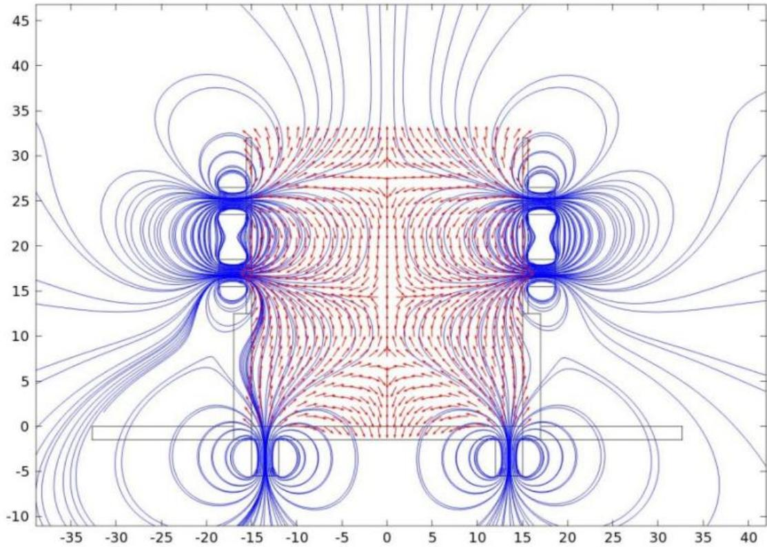
**Figure 2: Magnetic field design within a cylindrical ion thruster. This represents an axially symmetric model of the fields. The numbers provide a scale for size within the chamber, measured in mm. [3]**
