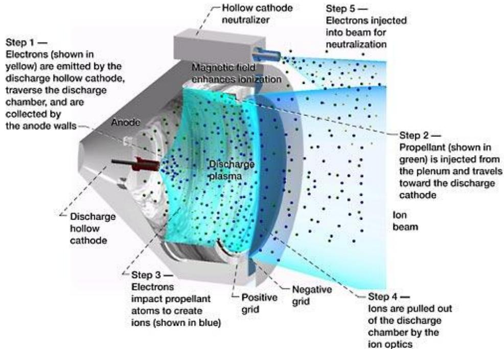
**Figure 1. Cutaway of an ion thruster depicting the components and steps of operation. [7].**
