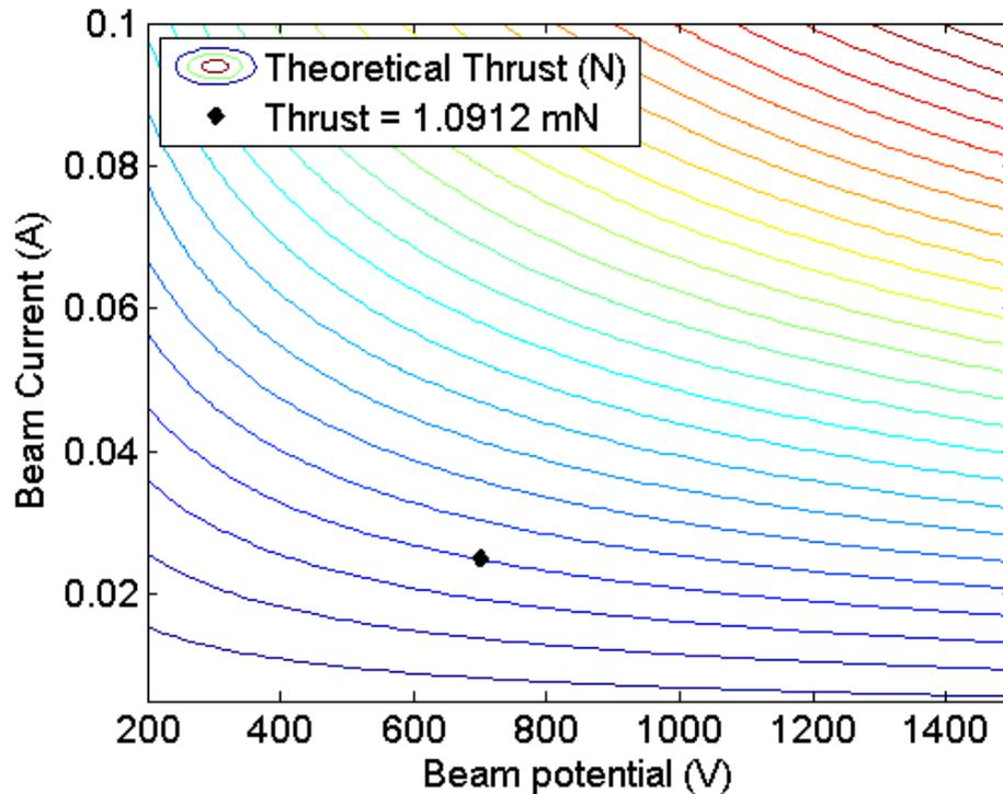
Figure 13: Thrust as a function of beam potential and beam current
