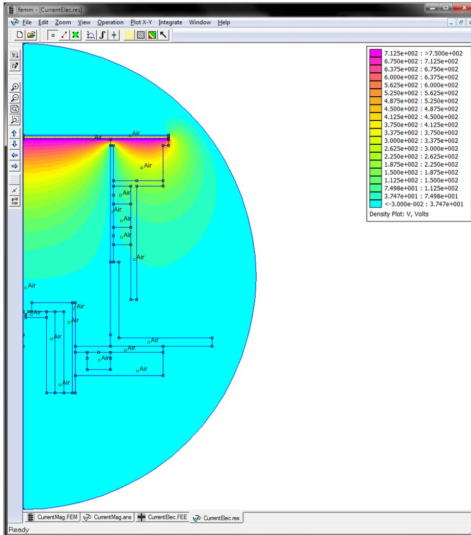
**Figure 10: Electrostatic solution of the ion thruster as calculated by FEMM.**
