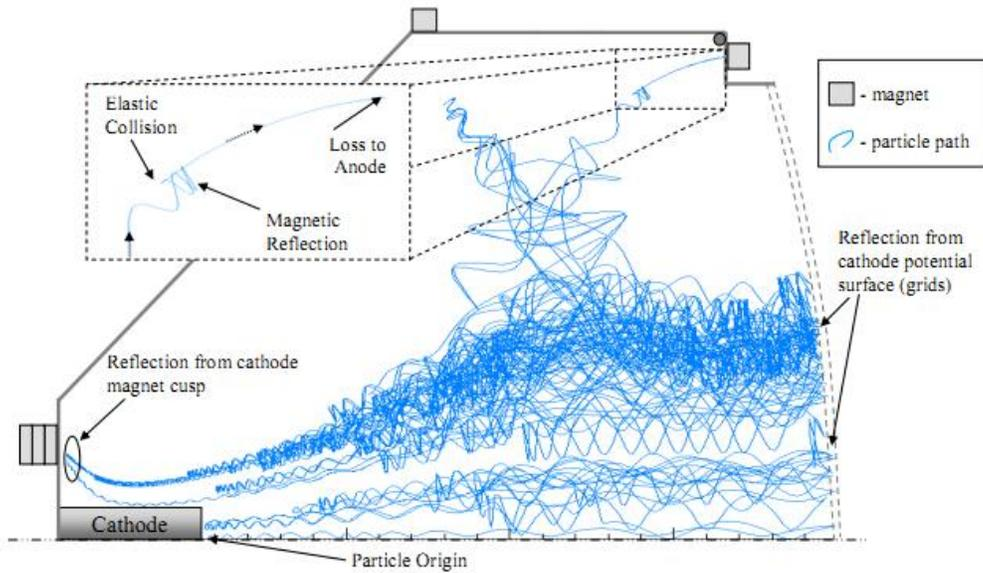
**Figure 3: Single electron motion within the ionization chamber. The electron is always contained within the ionization chamber. Important areas to pay attention to are the regions near the magnetic cusps. [1]**
