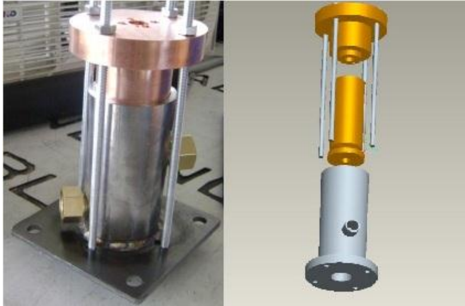
Figure 2. Injector plate, combustion chamber, cooling jacket. Assembled on left, exploded view on right. 2,3
