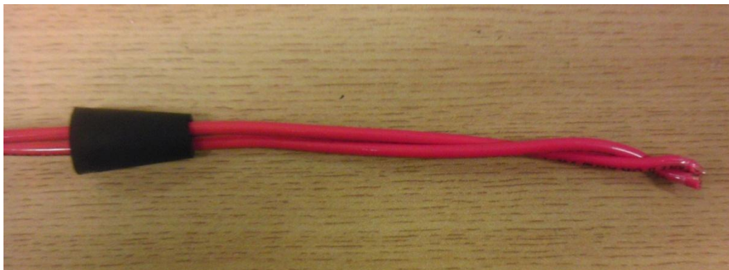
Figure 6. Igniter wires snaked through stopper, twisted together with stripped leads facing each other.
