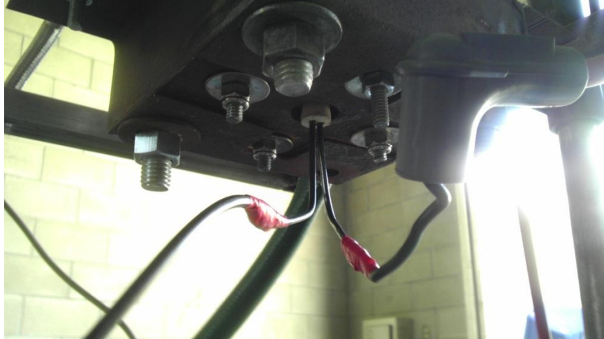
Figure 7. Igniter placed in nozzle exit, secured by stopper.
