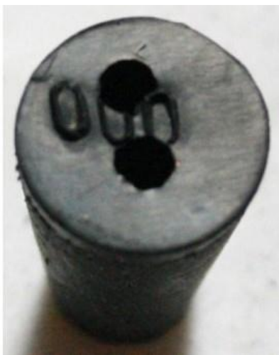
Figure 5. Size 000 rubber stopper, two preformed holes. 4
