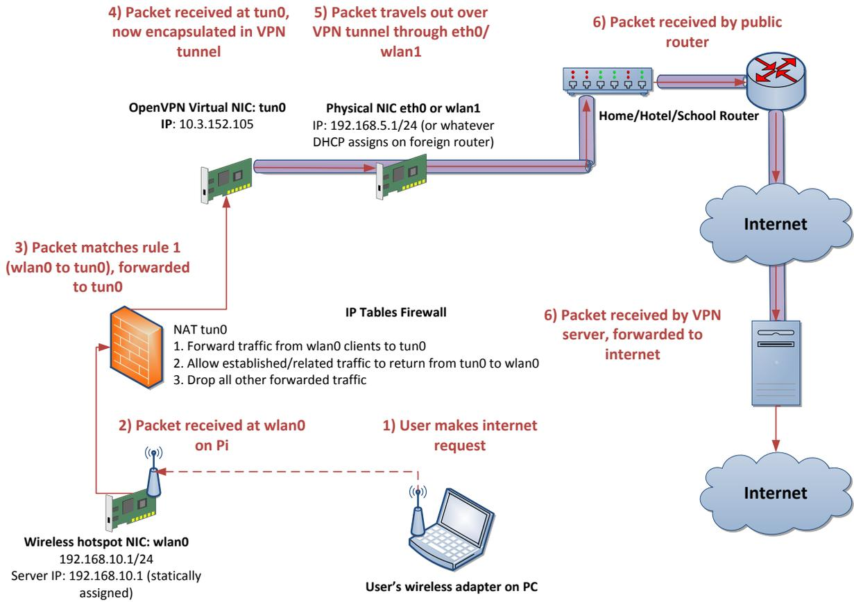
**Figure 4B: Tracing reply from internet back to secure hotspot client**
