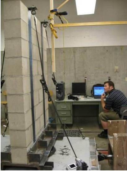
Master's student Joey Williams tests a fiber reinforced concrete masonry wall on the shake table as part of his project
