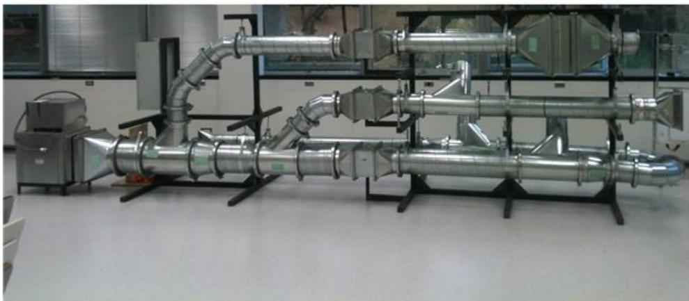
**Figure 2 Air Duct Simulator Schematic and Picture**
