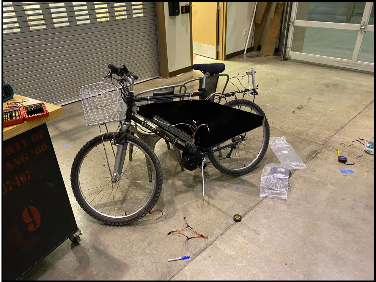
Installing battery/electrical system into the battery compartment.
