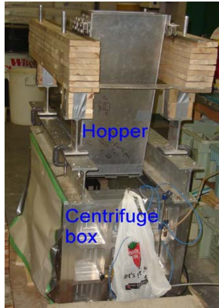
Figure 2. Setup for sand raining during test 2
