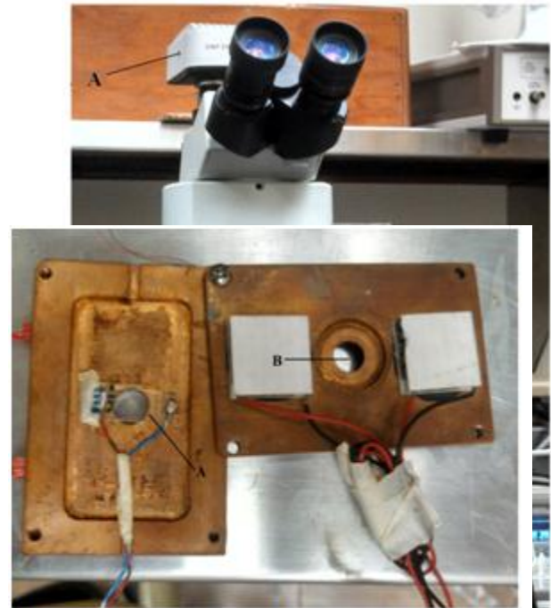
Figure 3: Oven along with a liquid crystal sample. A) Liquid crystal sample. B) Optical viewing port.
