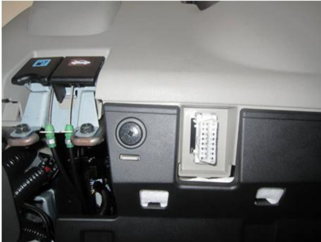
Figure 12 - OBD-II Port Location
