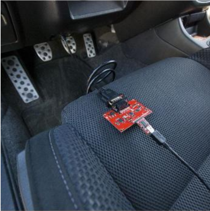
Figure 3 - Testing for CAN signals with a Sparkfun board
