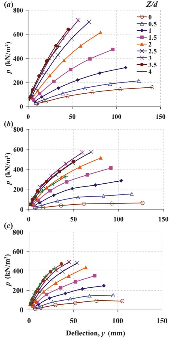
**Fig. 14.** Comparison of experimental  $p$ - $y$  curves for different loading angles -  $Z/d = 2$ .
