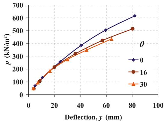
Fig. 15. Normalized  $p$ - $y$  curves for loading angles:  $0^\circ$ ,  $16^\circ$ , and  $30^\circ$ .
