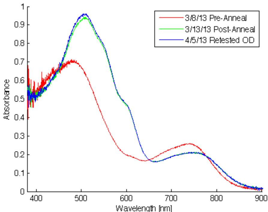
Figure 10: The optical effects of annealing on a 650 RPM polymer spun device.
