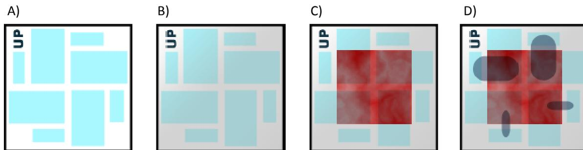
Figure 6: Demonstrating the step by step procedure to create a device. A) The cleaned substrate with patterned ITO, B) The PEDOT applied everywhere, C) The active layer applied and swabbed, D) The aluminum cathode applied to each pixel to complete the device.
