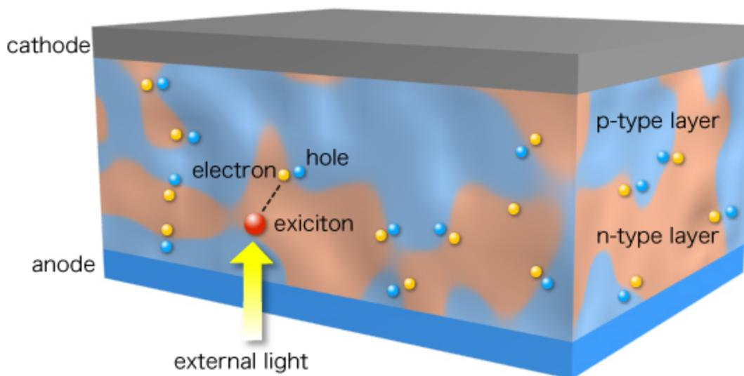
Figure 2: Bulk heterojunction containing p-type layer of active polymer and n-type layer of PCBM<sup>[9]</sup>.
