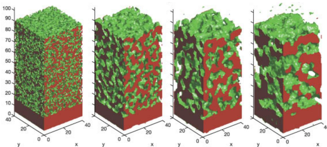
Figure 3: Changing morphology of the bulk heterojunction by annealing the devices. The left is the visualization of our solution when it is applied and the right is a visualization of a more ordered heterojunction<sup>[12]</sup>.
