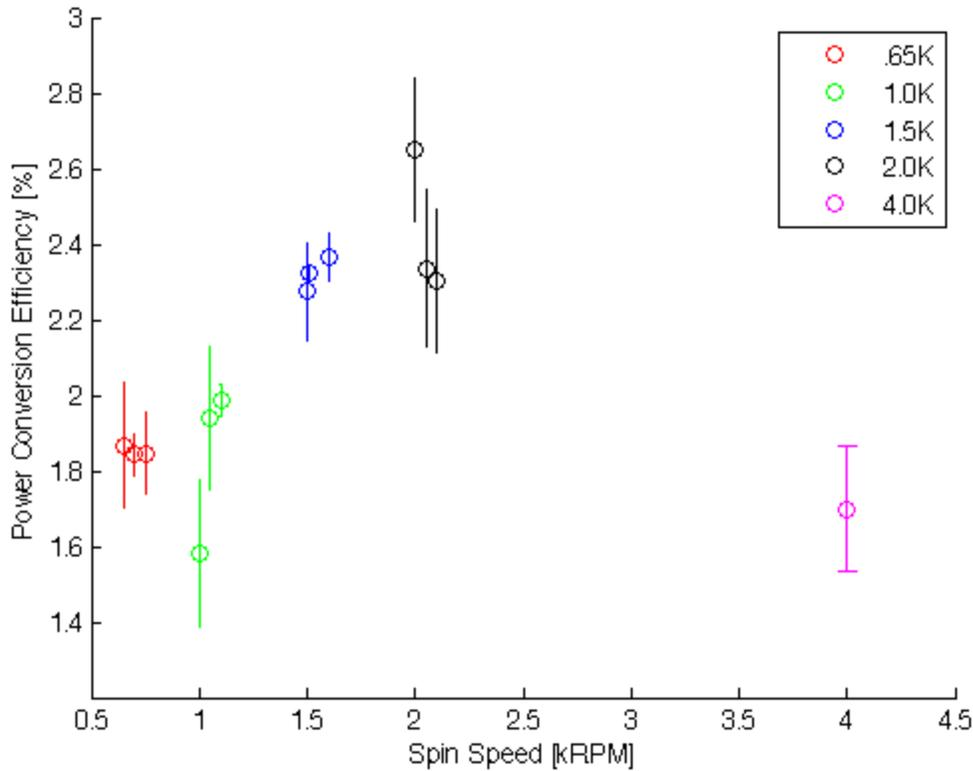
Figure 16: Power conversion efficiency dependency on spin speed. These measurements were taken for packaged devices illuminated in AM1.5 sunlight to consider realistic deployment conditions.
