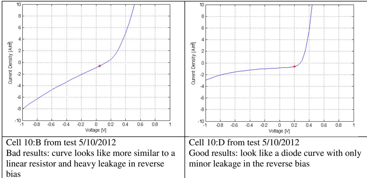
Figure 7: Qualitative pixel comparison to determine solar cell effectiveness
