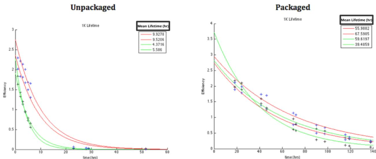
Figure 17: Importance of packaging and device sensitivity to atmospheric effects<sup>[15]</sup>
