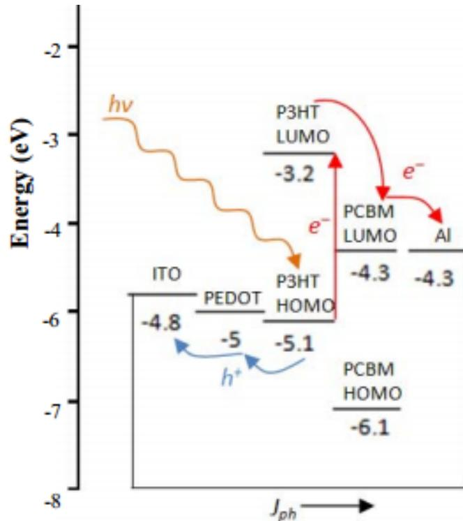
Figure 5: The energy level diagram of P3HT and PCBM in contact that illustrates the built in bias used to extract charge<sup>[13]</sup>.
