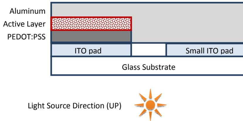
Figure 4: Device architecture
