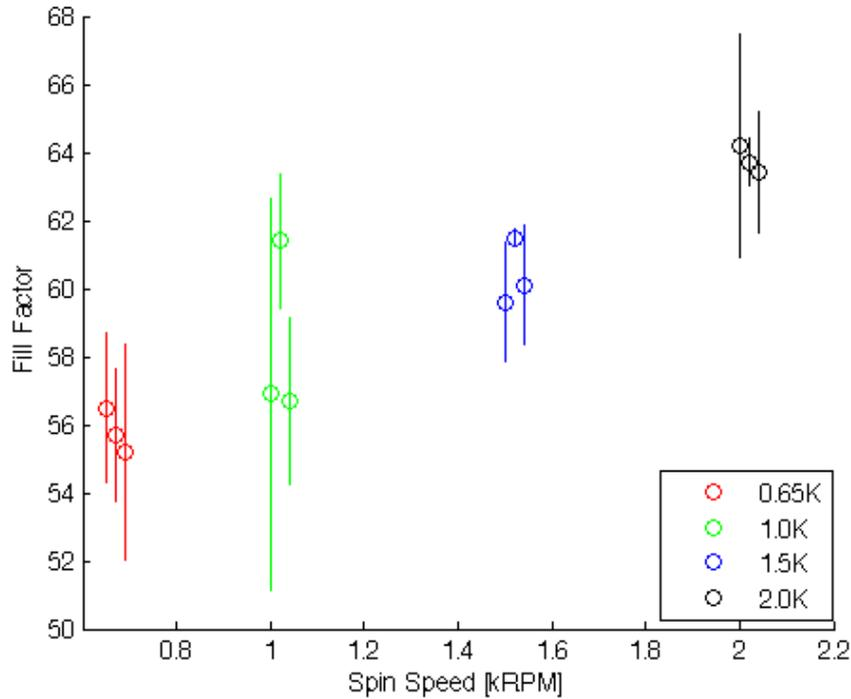
Figure 15: Fill factor dependency on thickness. These measurements were taken for packaged devices illuminated in AM1.5 sunlight to consider realistic deployment conditions. Uncertainties are the standard deviations between all pixels on a device
