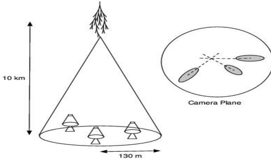
**Figure 2**<sup>[2]</sup>: The telescopes are positioned inside the light pool, the images from each telescope are combined to determine where the shower is coming from.
