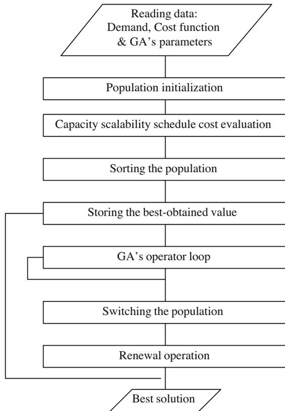
Fig. 1 Capacity scalability schedules generation using GAs
