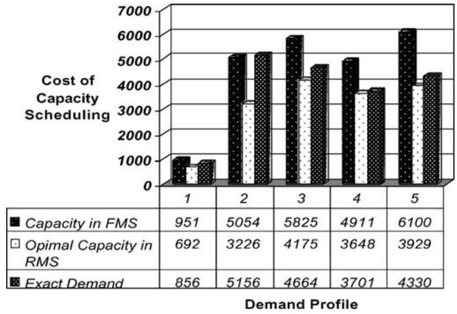
**Fig. 3** Cost of different capacity schedules at different demand profiles
