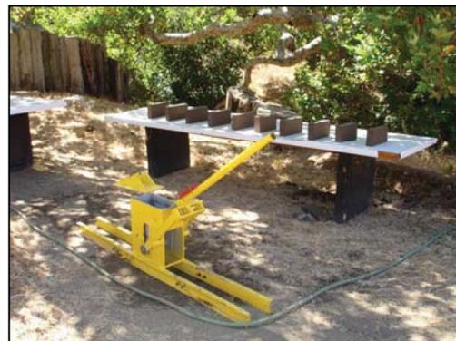
**Figure 2:** Hand brick press and bricks air curing.
