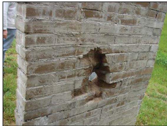
**Figure 10:** Single wythe wall and penetration, back face
