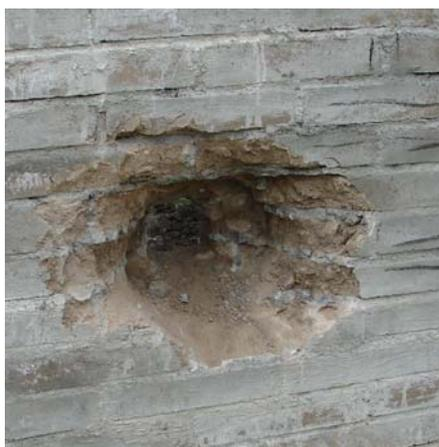
**Figure 13:** Double wythe wall and penetration by a chipping action of the hammer head, front face
