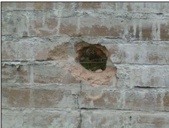
**Figure 9:** Single wythe wall and penetration, front face
