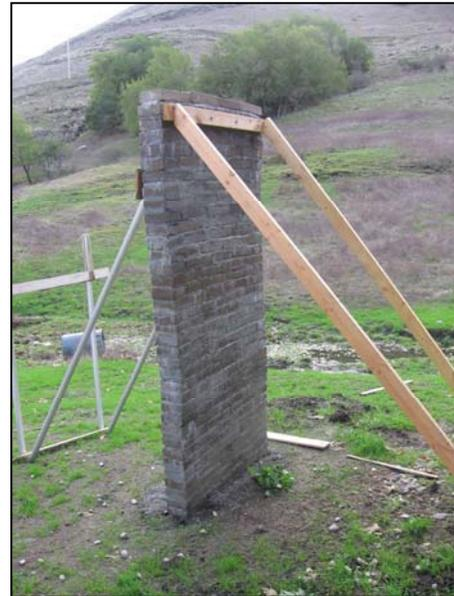
**Figure 6:** Flexible top of wall support
