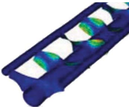
Fig. 7—Connecting plate deformation mode (755 Hz).
