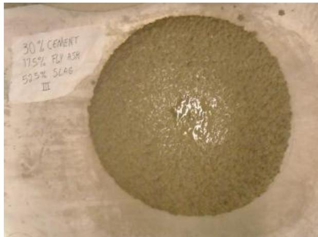
**Figure 1: Slump Flow Picture of 70SF Batch 3**
