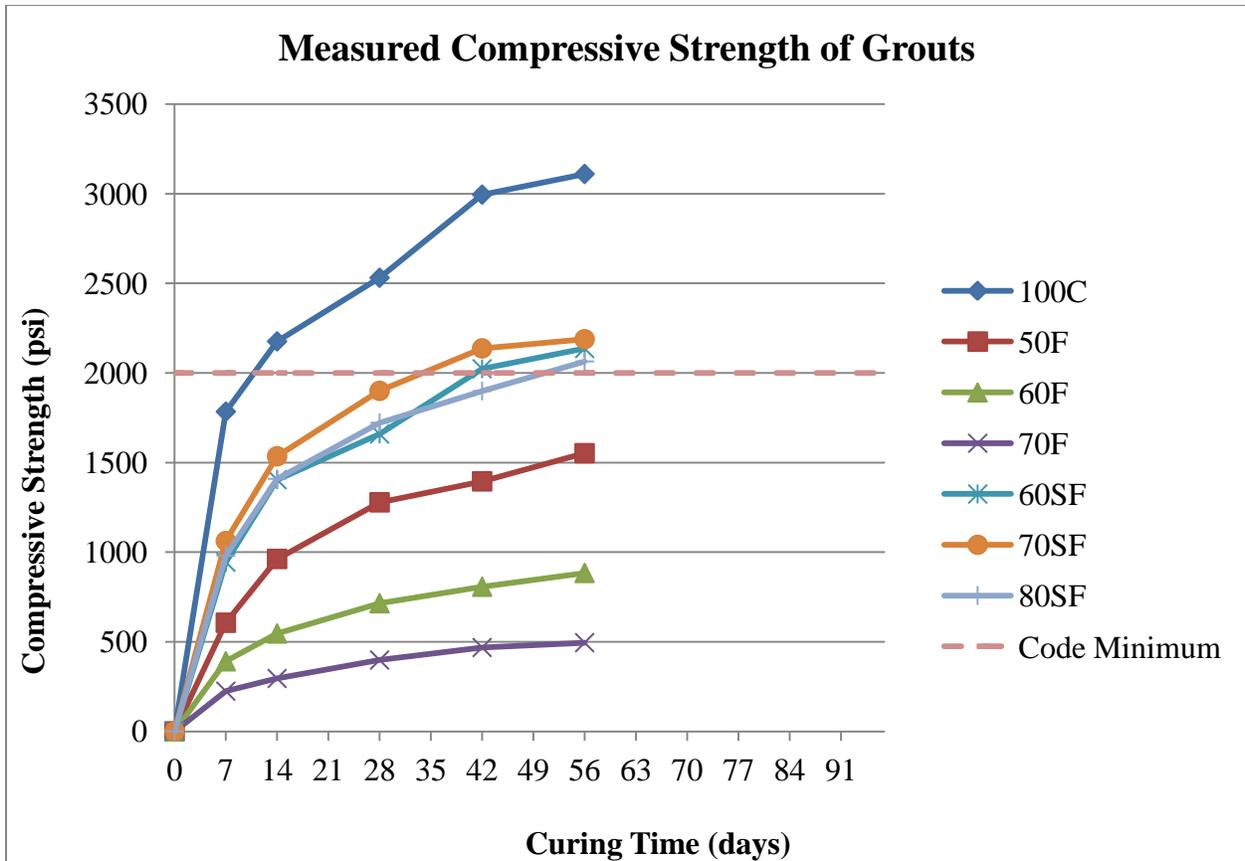
**Figure 12: Average Net Corrected Compressive Strength of Grouts**
