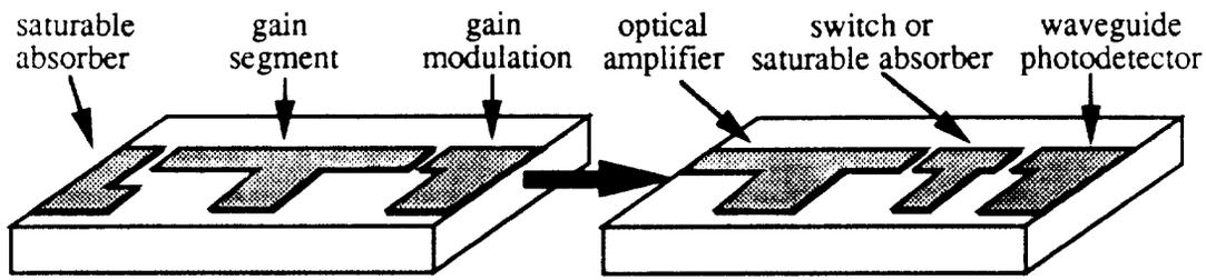
Fig. 1a. 3-section monolithic cavity mode-locked laser
