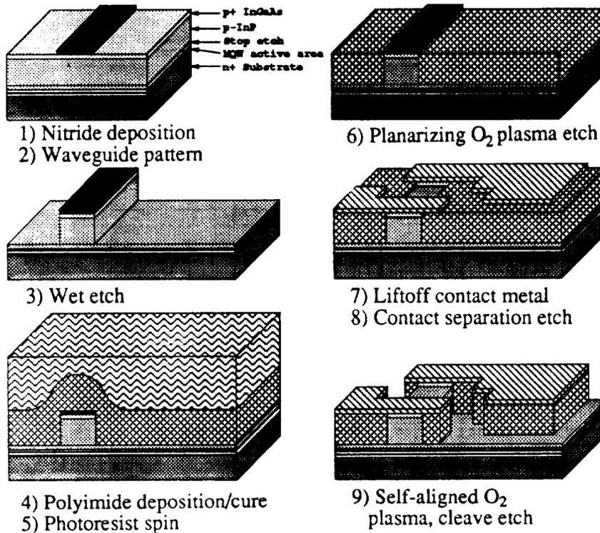
Fig. 4 . Low capacitance multi-section integration process
