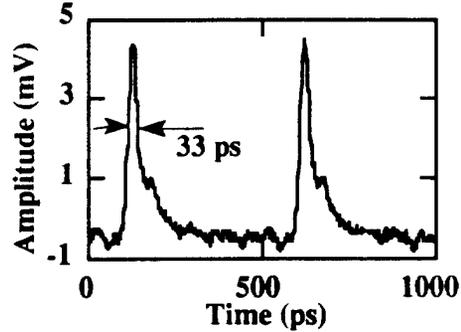
Fig. 3. Waveguide photodetector response
