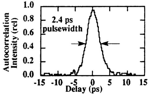
Fig. 2. Mode-locked laser autocorrelation
