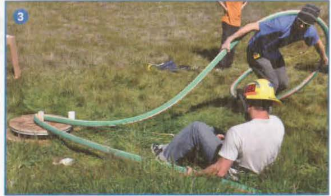
(2) A California Polytechnic State University fire protection engineering student conducts a test on nozzle forces that a firefighter would experience. (Photo by D.R. Turner.) (3) California Polytechnic State University fire protection engineering students conduct a test to measure hose kinking associated with CAFS. (Photo by D.R. Turner.)
