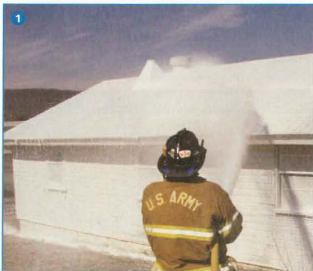
(1) When CAF is applied on a vertical surface, it can adhere to it for an extended time. (Photo by D. Madrzykowski.)
