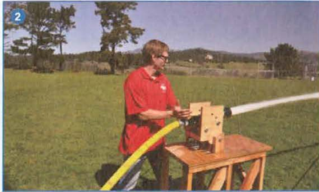
(2) A California Polytechnic State University fire protection engineering student conducts a test on nozzle forces that a firefighter would experience. (Photo by D.R. Turner.) (3) California Polytechnic State University fire protection engineering students conduct a test to measure hose kinking associated with CAFS. (Photo by D.R. Turner.)
