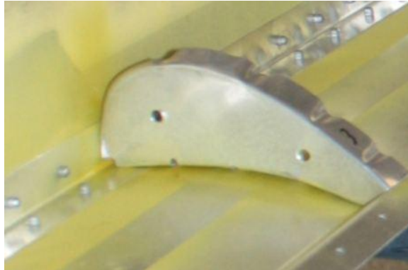
Figure 4. The inside of a slat, showing the Zinc Chromate (yellow) between the two surfaces.
