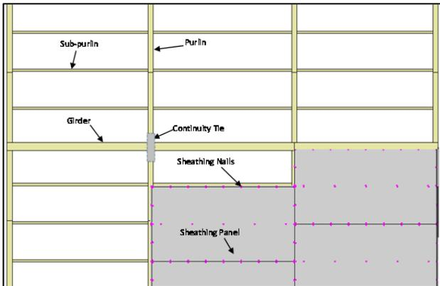
Figure 5. A section of a panelized roof diaphragm.
