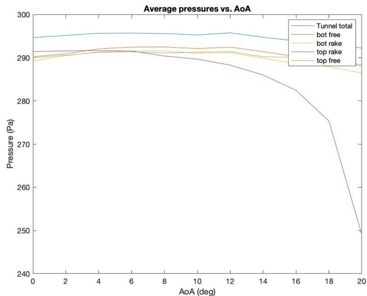
**Pressure data collected from the drag rake prototype during wind tunnel testing. The trend of decreasing pressure with increased AoA (angle of attack) is apparent and expected.**
