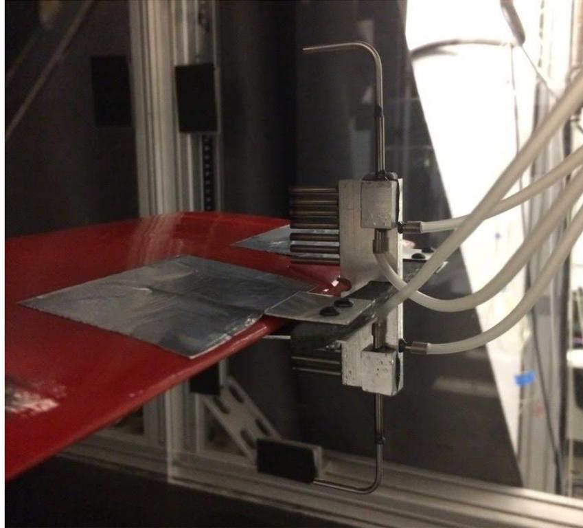
**The first drag rake prototype and mount prototype in the wind tunnel.**
