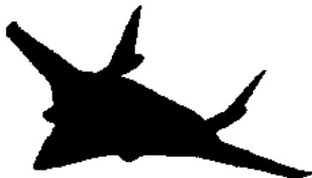
Figure 3. Configuration 3 is a complete blended wing body with embedded engines.
