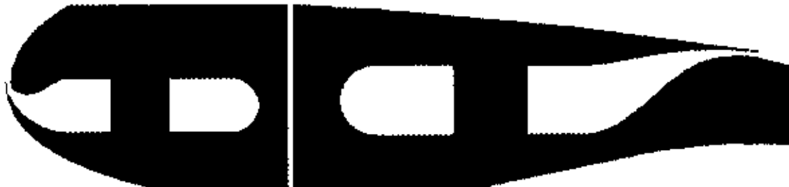
Figure 11. A schematic showing the cross section of (a) the leading and (b) the trailing edge plenums highlighting the meat foam flow straightener placement.
