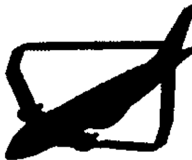
Figure 4. Configuration 4 utilizes a high aspect ratio wing, in a diamond wing configuration.
