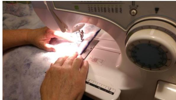
*Figure 45. Backing of quilt-style fabric sheet being sewn*
