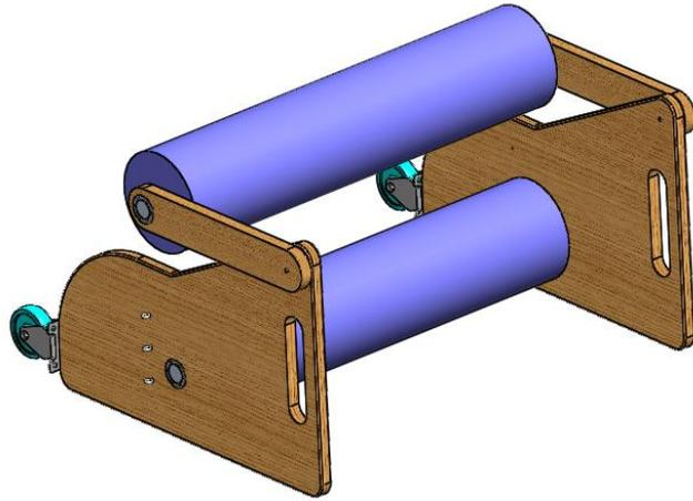
Figure 12. Pressure Applicator Concept - Single Squeezer Built by Team
