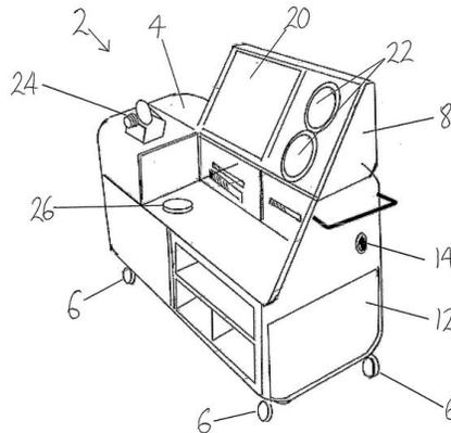
Figure 3. Patented Sensory Apparatus for the mobile transport of sensory items in hospitals
