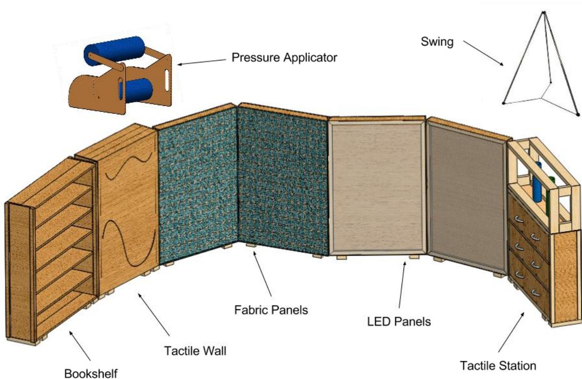
Figure 14. Labeled Room Components
