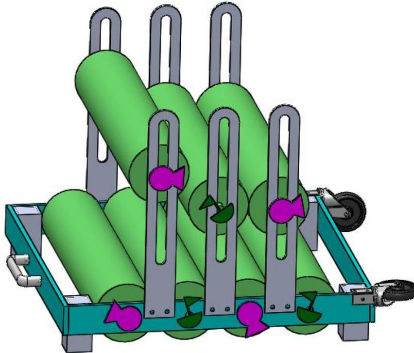
Figure 9. Pressure Applicator Concept: Squeeze Tunnel
