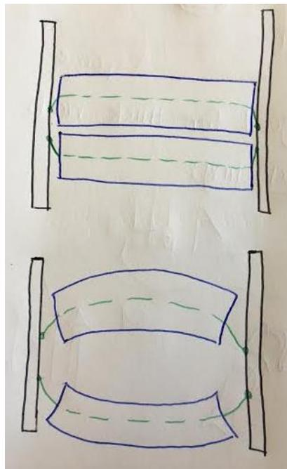
Figure 13. Pressure Applicator Concept - Loose Bungee
