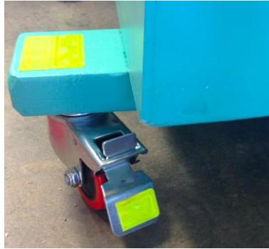
Figure 18. Lockable casters on panel walls with reflective yellow safety strips.
