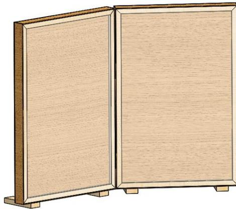
*Figure 25. Solidworks model of the LED panels (casters not shown)*
