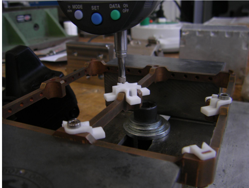
Figure 9: A full frame halfway through a cycle. The arm begins by zeroing on the raised frame next to the small spacer and working its way around the frame counterclockwise.
