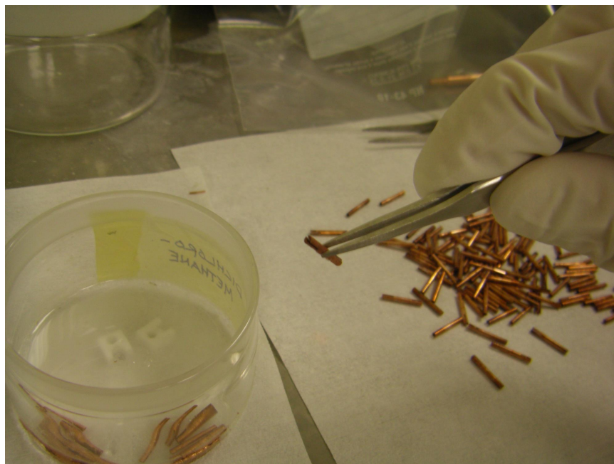
Figure 7: The set up for cleaning the epoxy off of the copper pins. The pins to be cleaned can be seen on the right, and the glass container on the left contains the pins soaking in the dichloromethane.
