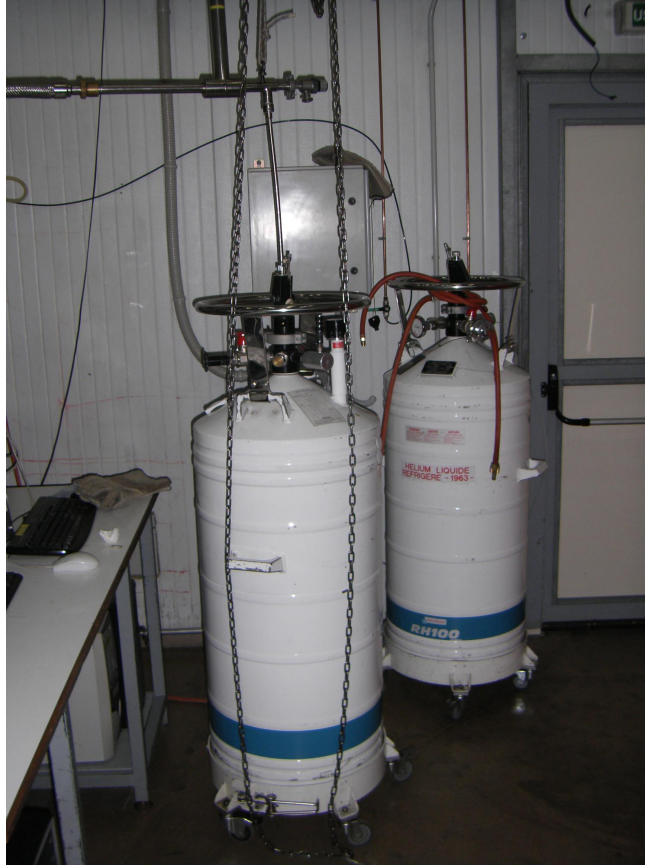
Figure 4: Liquid Helium Dewar being used to fill the main bath. The pipe coming out of the top is connected to the top of the cryostat which allows the main bath to be filled.
