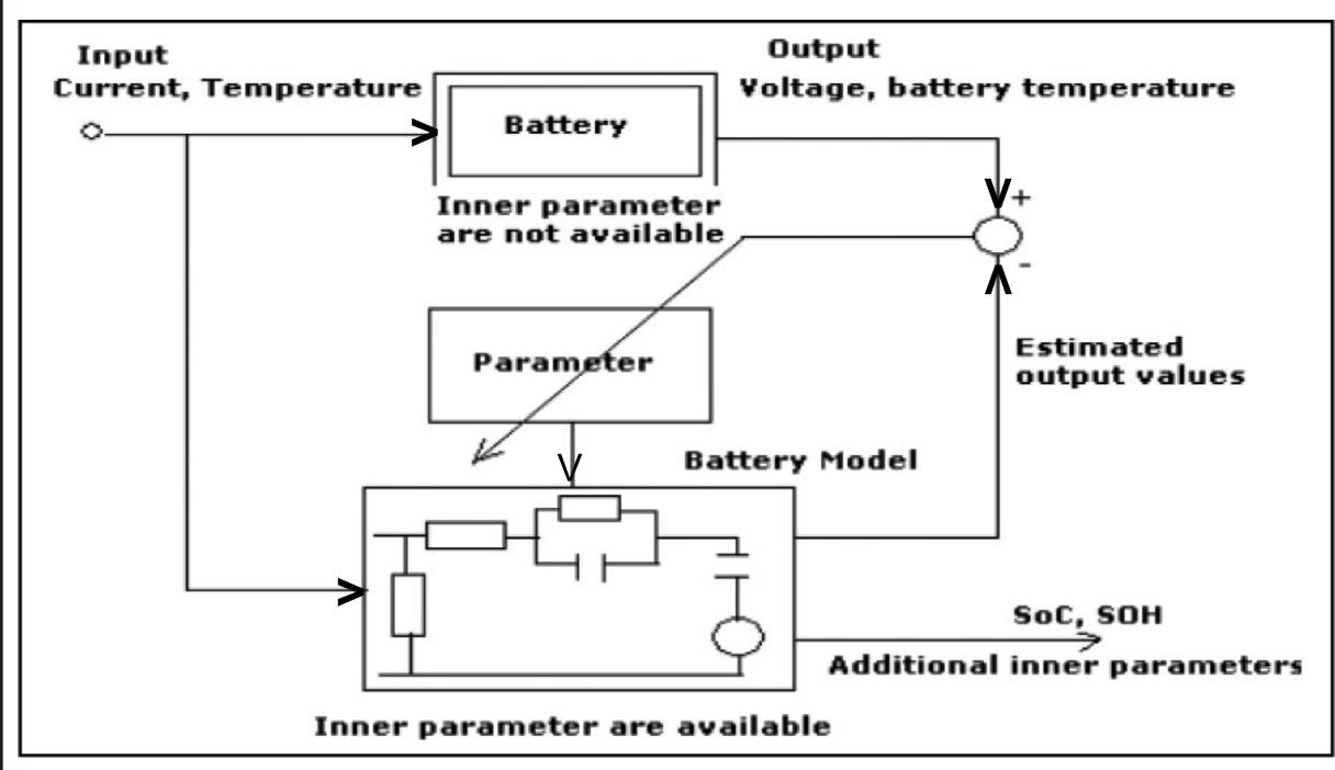
RSOC determination using Kalman filter.
