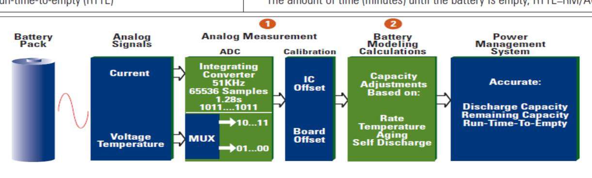
The two components of battery fuel gauge accuracy depend on analog measurement and battery modeling.
