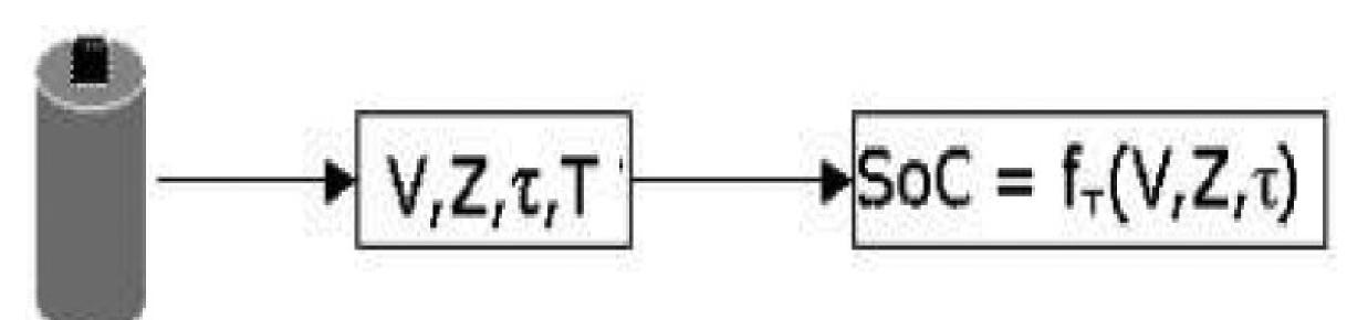
Where SoC is state of charge, and the variables such as battery voltage (V), battery impedance (Z), and the voltage relaxation time (τ)
