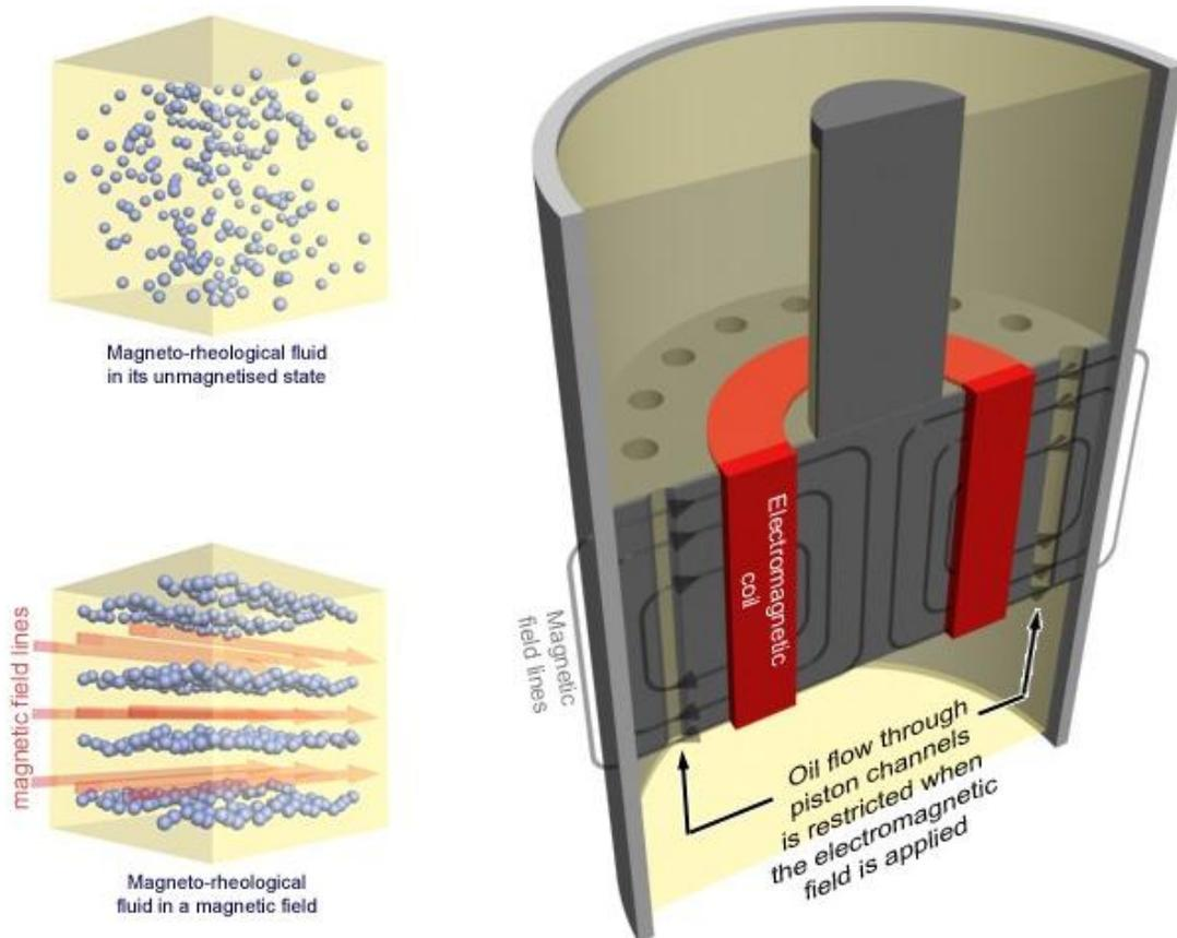
**Figure 5:** MagneRide Suspension Cutaway<sup>vi</sup>
