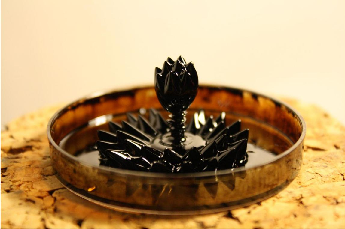
**Figure 1:** An ordinary wood screw coated in Ferro fluid with a permanent neodymium magnet underneath.
