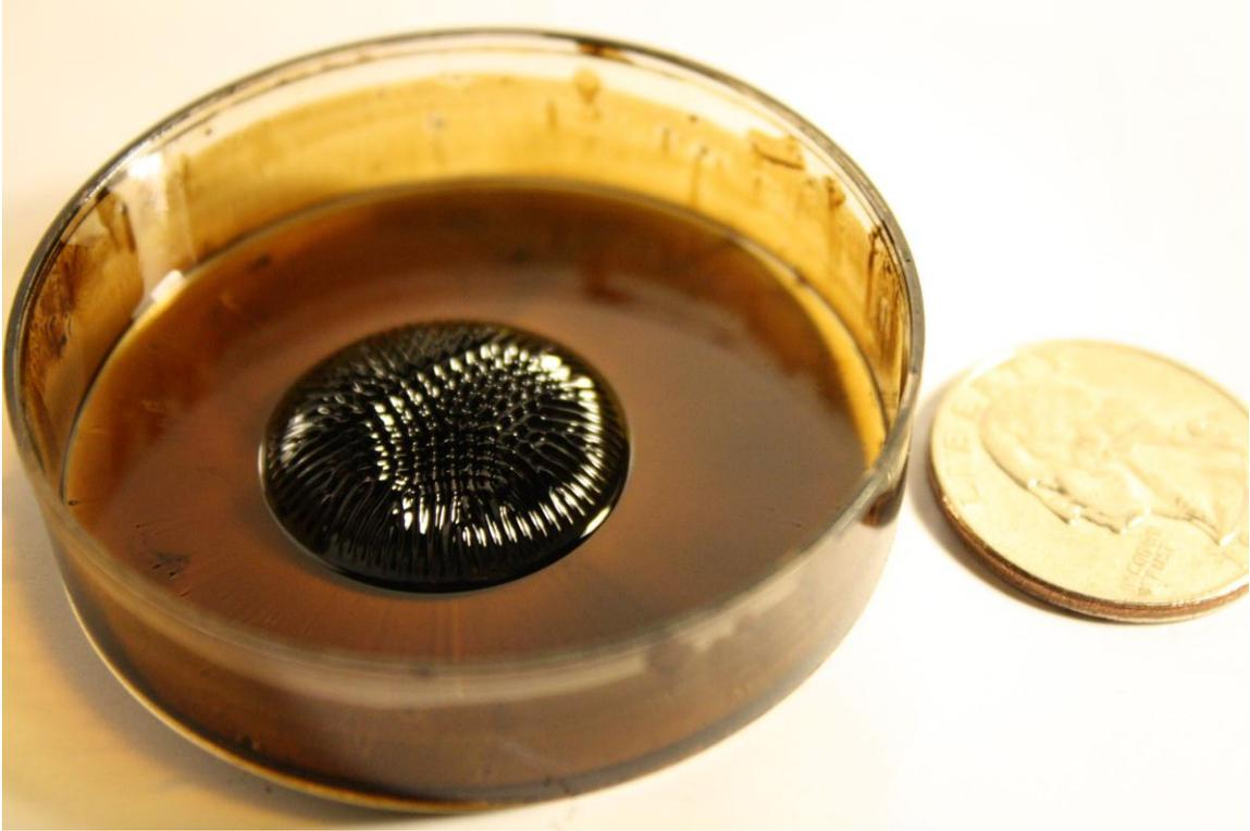
**Figure 2:** Ferro fluid under a strong magnetic field. In this case a rare earth neodymium magnet has been placed directly below the container. One can notice the more numerous yet smaller protrusions. A US quarter is used for scale. Photo by Richard Kwok.
