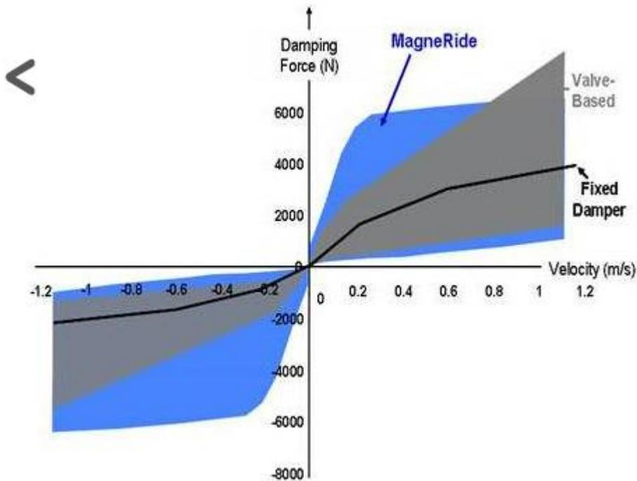
**Figure 6:** MagneRide compared to conventional dampeners<sup>viii</sup>
