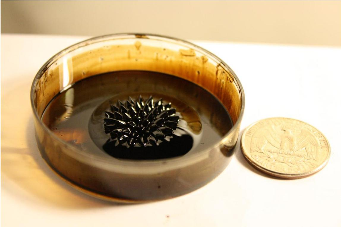
**Figure 3:** Ferro fluid under a slightly weaker magnetic field. The same permanent magnet with the same amount of fluid but the magnet is now separated from the container by half a centimeter. Notice that the protrusions are larger and less numerous. Photo by Richard Kwok.
