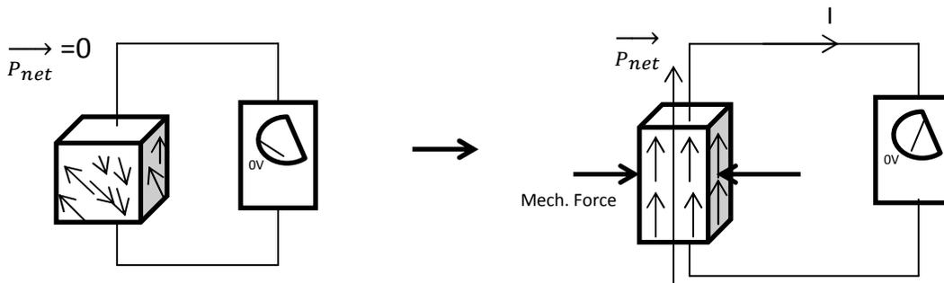
Figure 1: A piezoelectric material generates a voltage when a mechanical force is applied to it in the just the right way to align dipoles and/or move ions in the solid.
